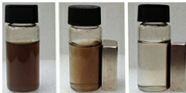
Fig. 1. Magnetic separation of nanoadsorbent from treated water
