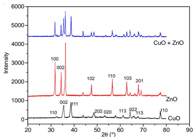
Fig. 1a. Combined powder X-ray diffraction pattern of CuO nanoparticles, ZnO nanoparticles and bimetallic Cu-Zn oxide nanoparticles
