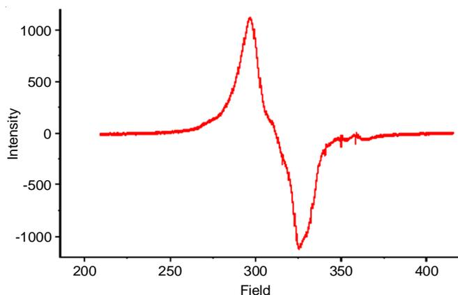
Fig. 3a. ESR spectra of Cu-Zn oxide nanoparticles
