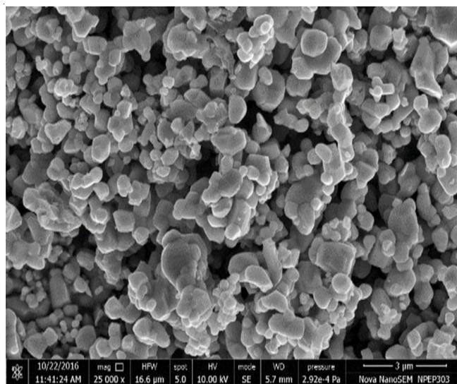
Fig. 2a. FE-SEM image of Cu-Zn oxide nanoparticles
