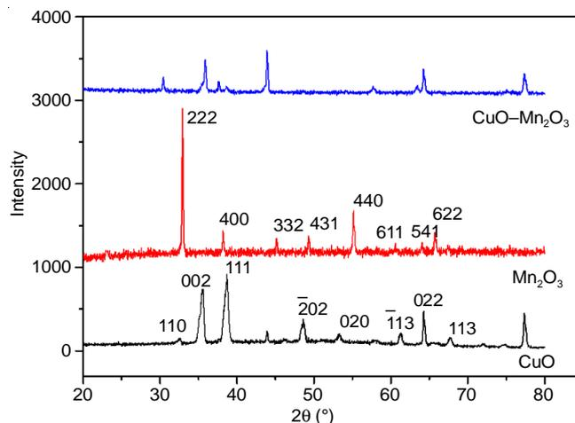
Fig. 1b. Combined powder X-ray diffraction pattern of CuO nanoparticles, MnO nanoparticles and bimetallic Cu-Mn oxide nanoparticles
