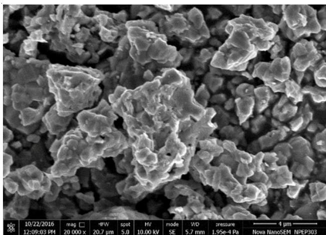
Fig. 2b. FE-SEM image of Cu-Mn oxide nanoparticle
