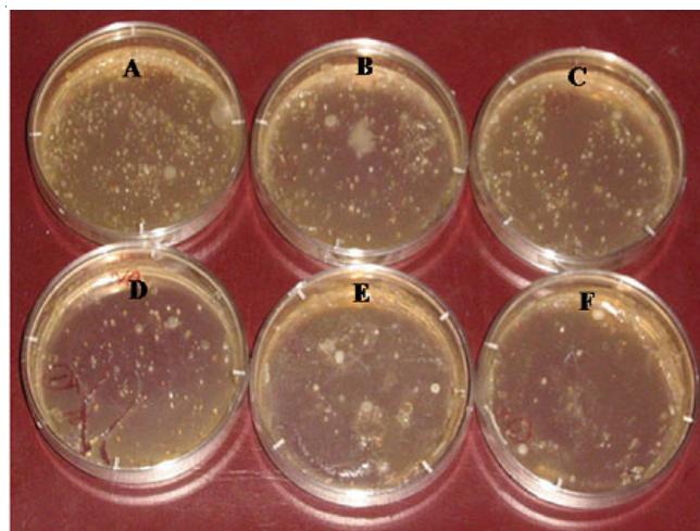
Fig. 9. Micrograph of biogrowth on Al-Zn anode with different amounts of NiO incorporation under natural marine conditions (A) 0%, (B) 0.05%, (C) 0.1%, (D) 0.2%, (E) 0.5%, (F) 1%
