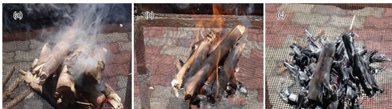
Fig. 1. Photo of combustion stages, (a) smouldering combustion; (b) flaming combustion and (c) charring combustion
