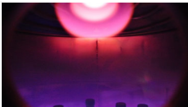
Fig. 4. Plasma generated in the vacuum chamber during treatment of sealed bottles with ultra-pure water. On the top the cathode glow (ion source). Below the glow of plasma surrounding the bottles with liquid
