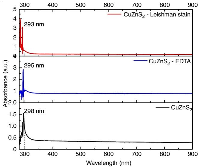
Fig. 5. Optical absorbance (A) of the as deposited films CuZnS<sub>2</sub>, CuZnS<sub>2</sub> with EDTA added and CuZnS<sub>2</sub> with Leishman stain added
