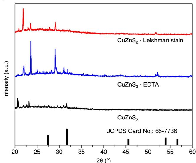
Fig. 1. X-ray diffraction patterns of as-grown CuZnS<sub>2</sub> films, CuZnS<sub>2</sub> with EDTA and Leishman stain added
