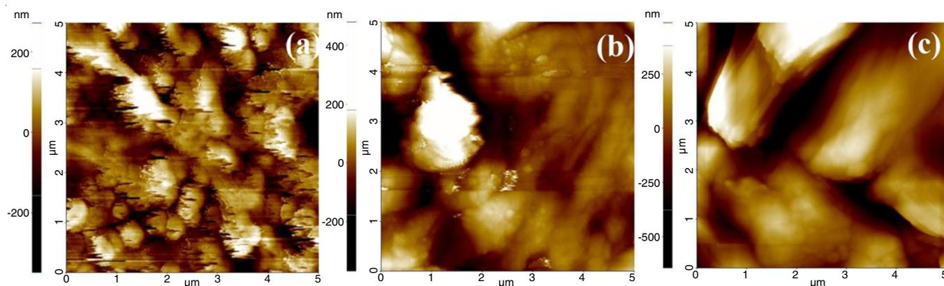
Fig. 4. AFM 2D images of the as grown films (a)  $\text{CuZnS}_2$ , (b)  $\text{CuZnS}_2$  with EDTA added and (c)  $\text{CuZnS}_2$  with Leishman stain added
