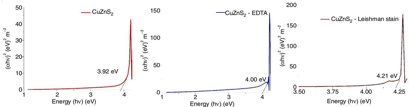
Fig. 6. Band gap of the prepared films CuZnS<sub>2</sub>, CuZnS<sub>2</sub> with EDTA added and CuZnS<sub>2</sub> with Leishman stain added
