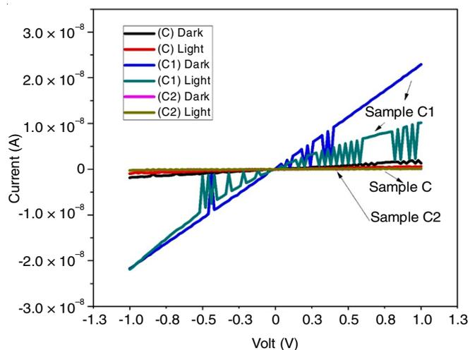
Fig. 7. I-V characteristics for the samples C, C1, C2 films for CuZnS<sub>2</sub>, CuZnS<sub>2</sub> with EDTA added and CuZnS<sub>2</sub> with Leishman stain added
