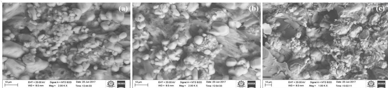
Fig. 2. Scanning electron microscopic images of as-grown films (a)  $\text{CuZnS}_2$ , (b)  $\text{CuZnS}_2$  with EDTA added and (c)  $\text{CuZnS}_2$  with Leishman stain added
