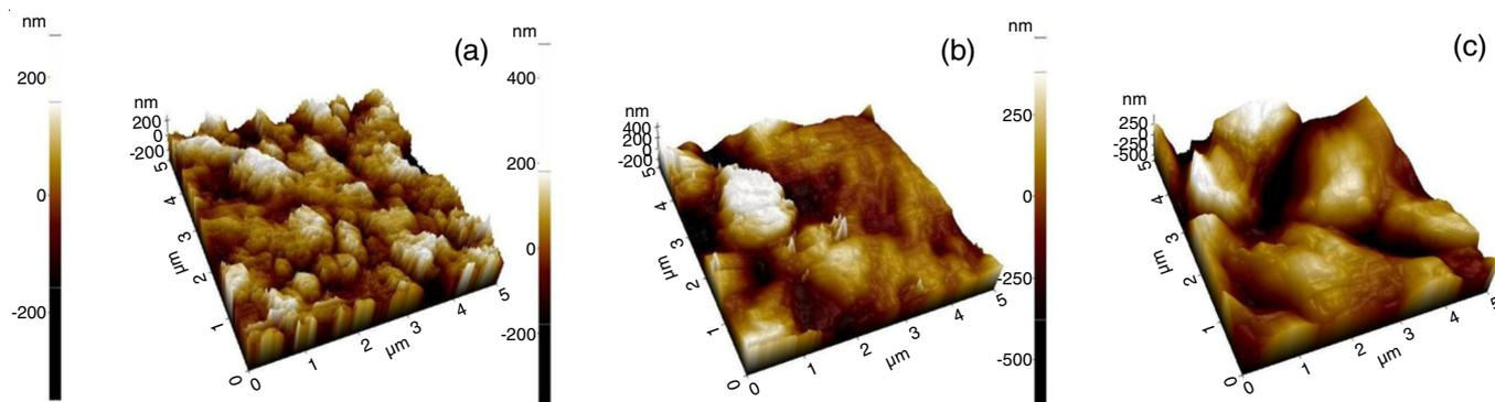
Fig. 3. AFM 3D images of the as deposited films (a)  $\text{CuZnS}_2$ , (b)  $\text{CuZnS}_2$  with EDTA added and (c)  $\text{CuZnS}_2$  with Leishman stain added
