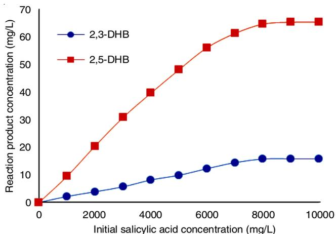
Fig. 3. Concentration of salicylic acid decomposition products at 0.5 h
