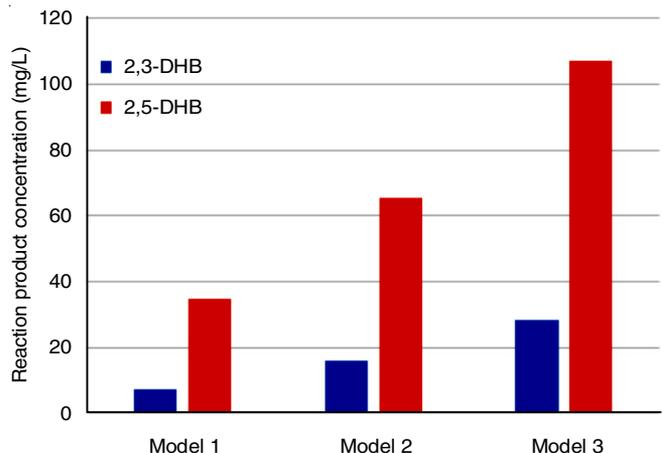
Fig. 5. Concentration of salicylic acid decomposition products in different plasma modes
