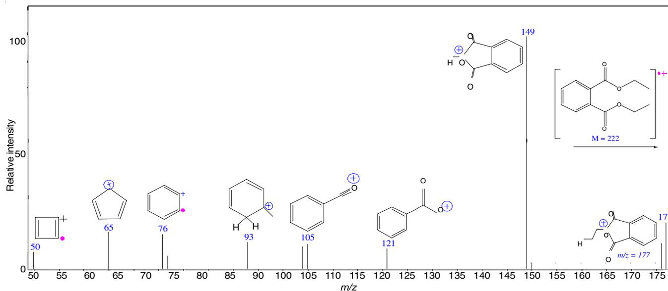
Fig. 2. Mass spectrum and fragmentation of diethyl phthalate
