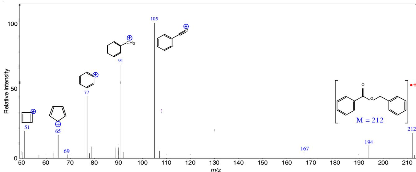
Fig. 1. Mass spectrum and fragmentation of benzyl benzoate
