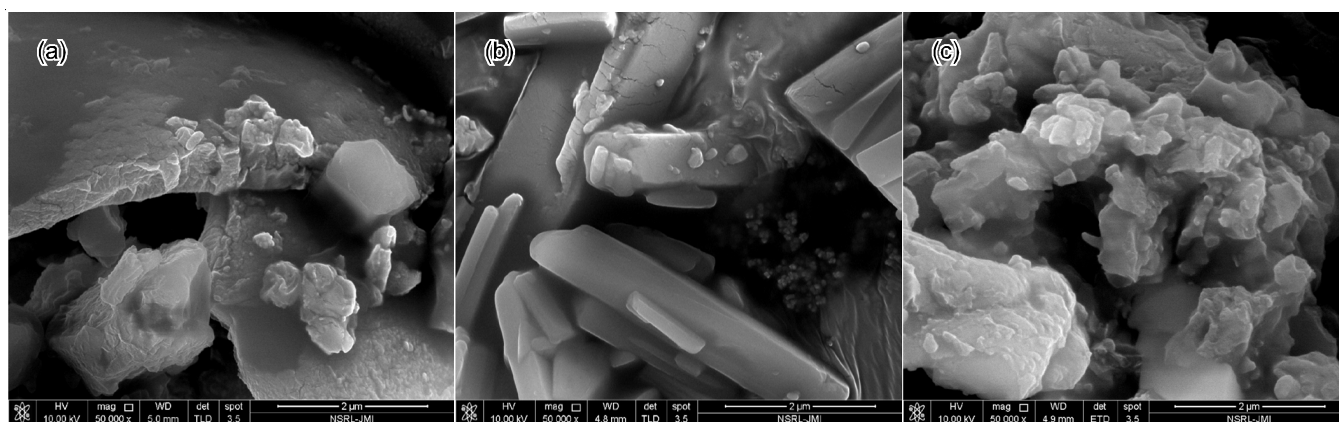
Fig. 3. SEM images of NGB + EDTA (a); JGB + EDTA (b) and NGB + JGB + EDTA systems (c)
