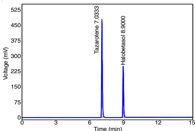
Fig. 4b. Chromatogram of standard solution of halobetasol and tazarotene
