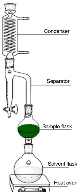
Fig. 1. System of the lemon peels essential oil extraction by the steam distillation method
