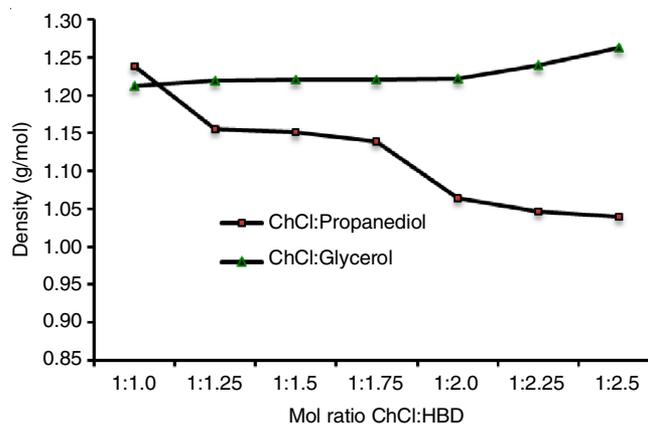
Fig. 1. Effect of molar ratio ChCl:HBD to DES density
