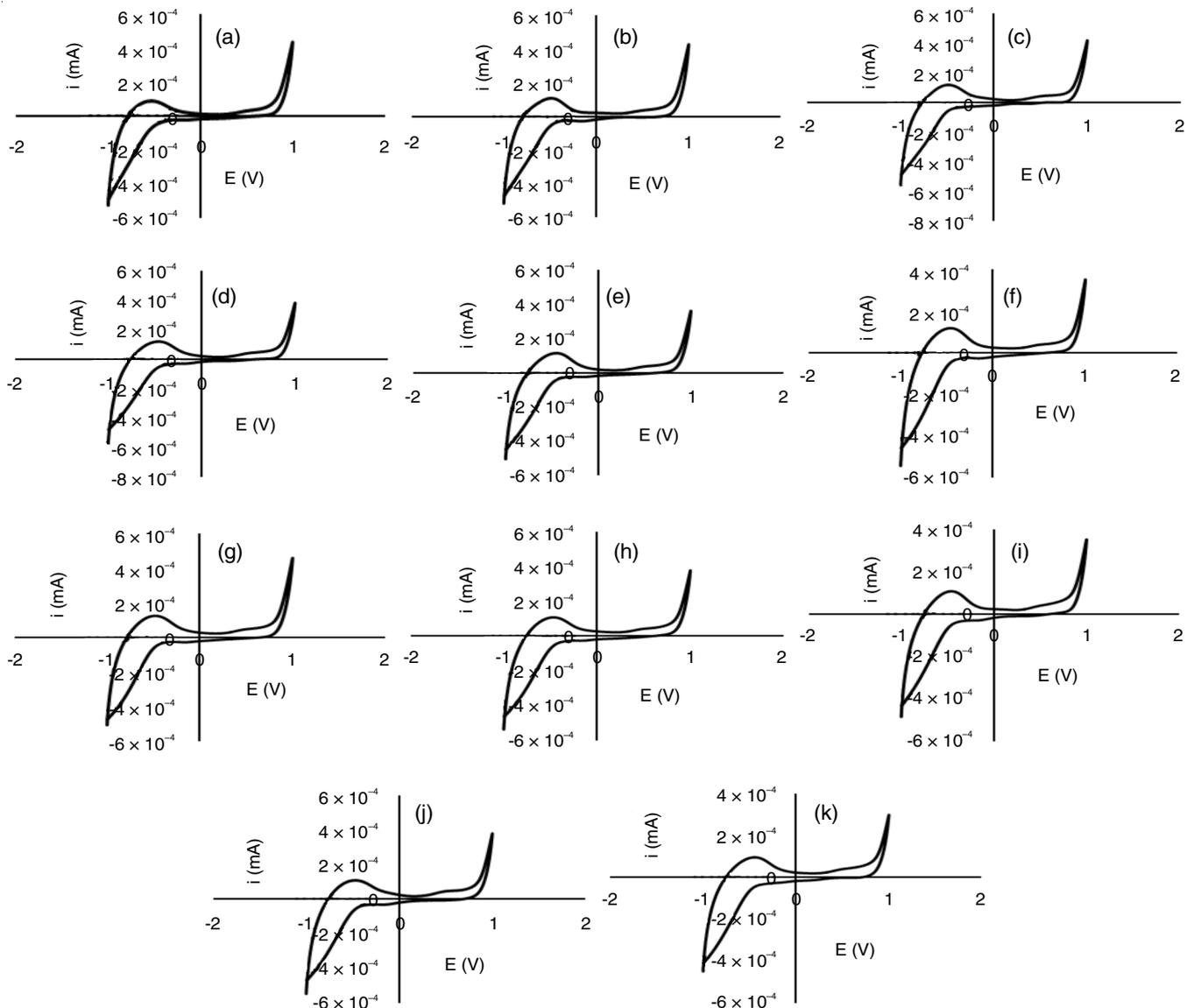
Fig. 3. Voltammograms of stainless steel on water electrolysis in the fermented flour 0-10 g/L addition (a-k) and base condition
