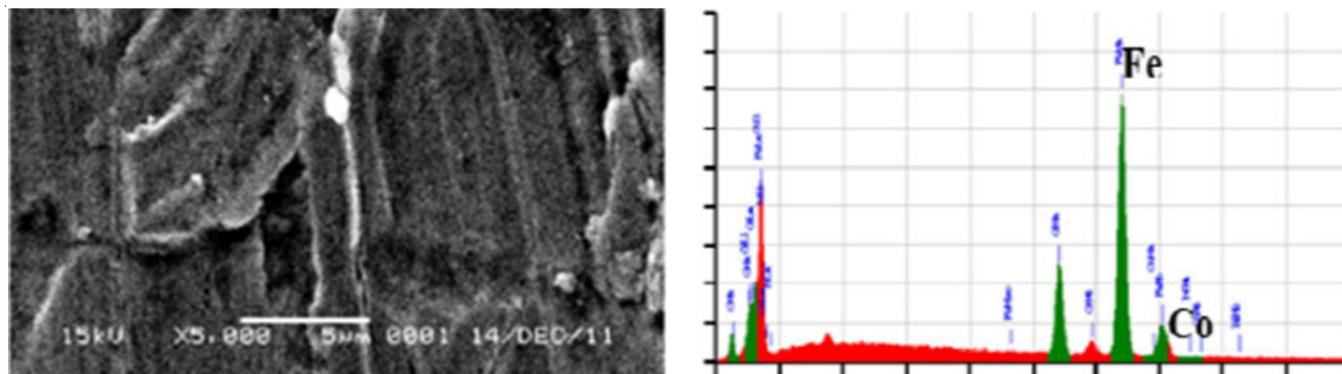
Fig. 1. SEM-EDAX spectrum of stainless steel
