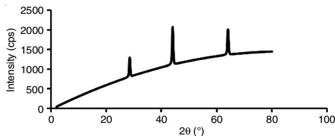
Fig. 2. XRD spectrum of stainless steel
