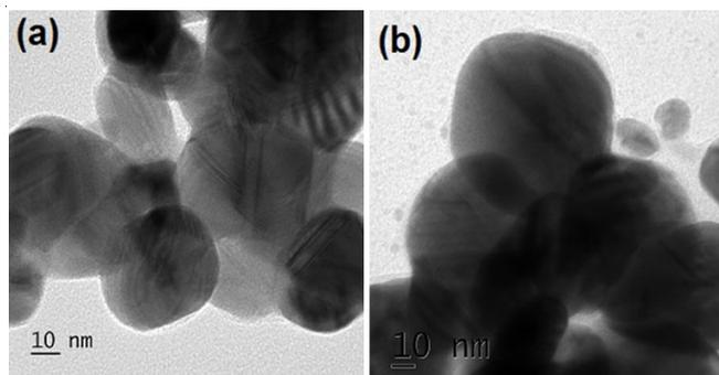
Fig. 3. TEM micrograph of (a) AgNP-C and (b) AgNP-B
