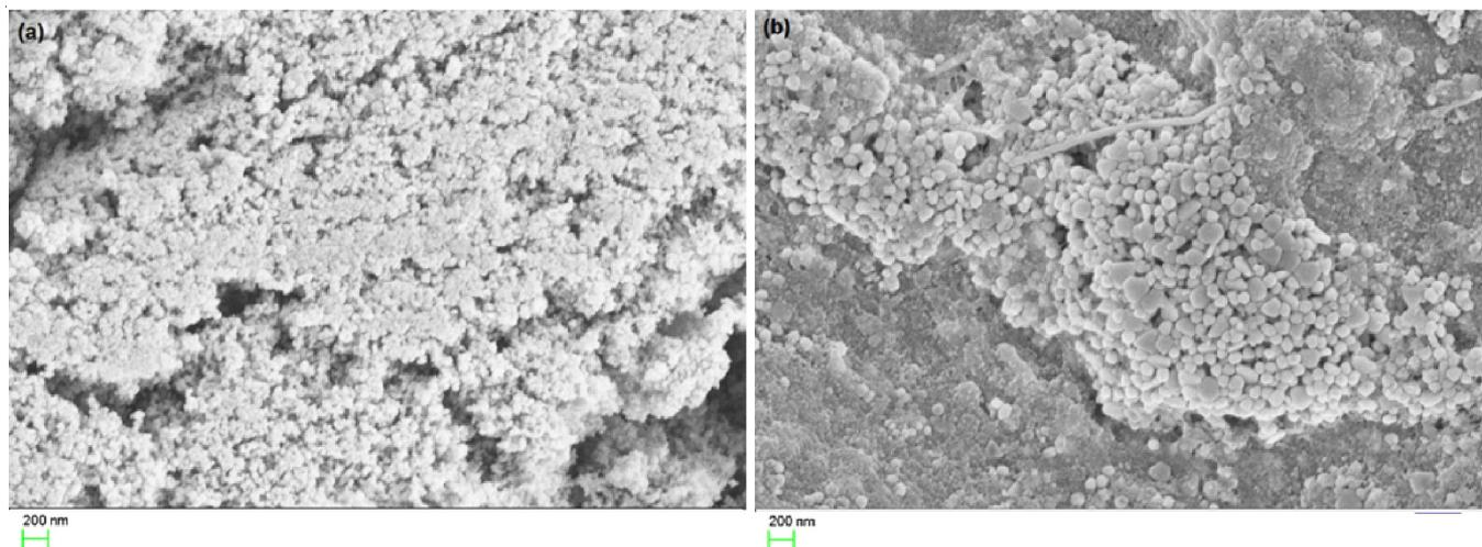
Fig. 2. SEM micrograph of (a) AgNP-C and (b) AgNP-B
