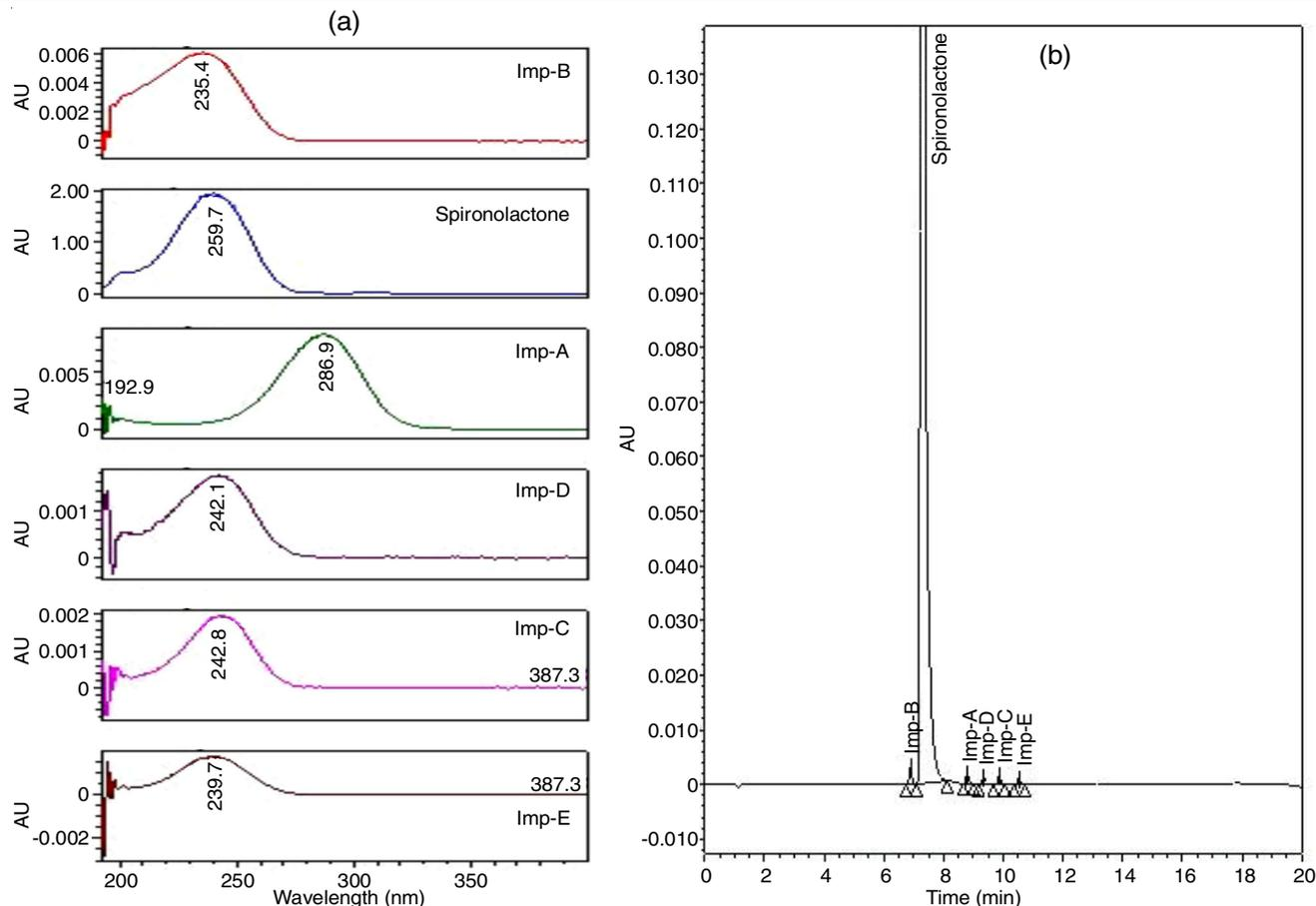
Fig. 2. (a) UV overlay spectra of spironolactone and its impurities A, B, C, D and E; (b) Chromatogram of spironolactone and its impurities A, B, C, D and E in final chromatographic conditions
