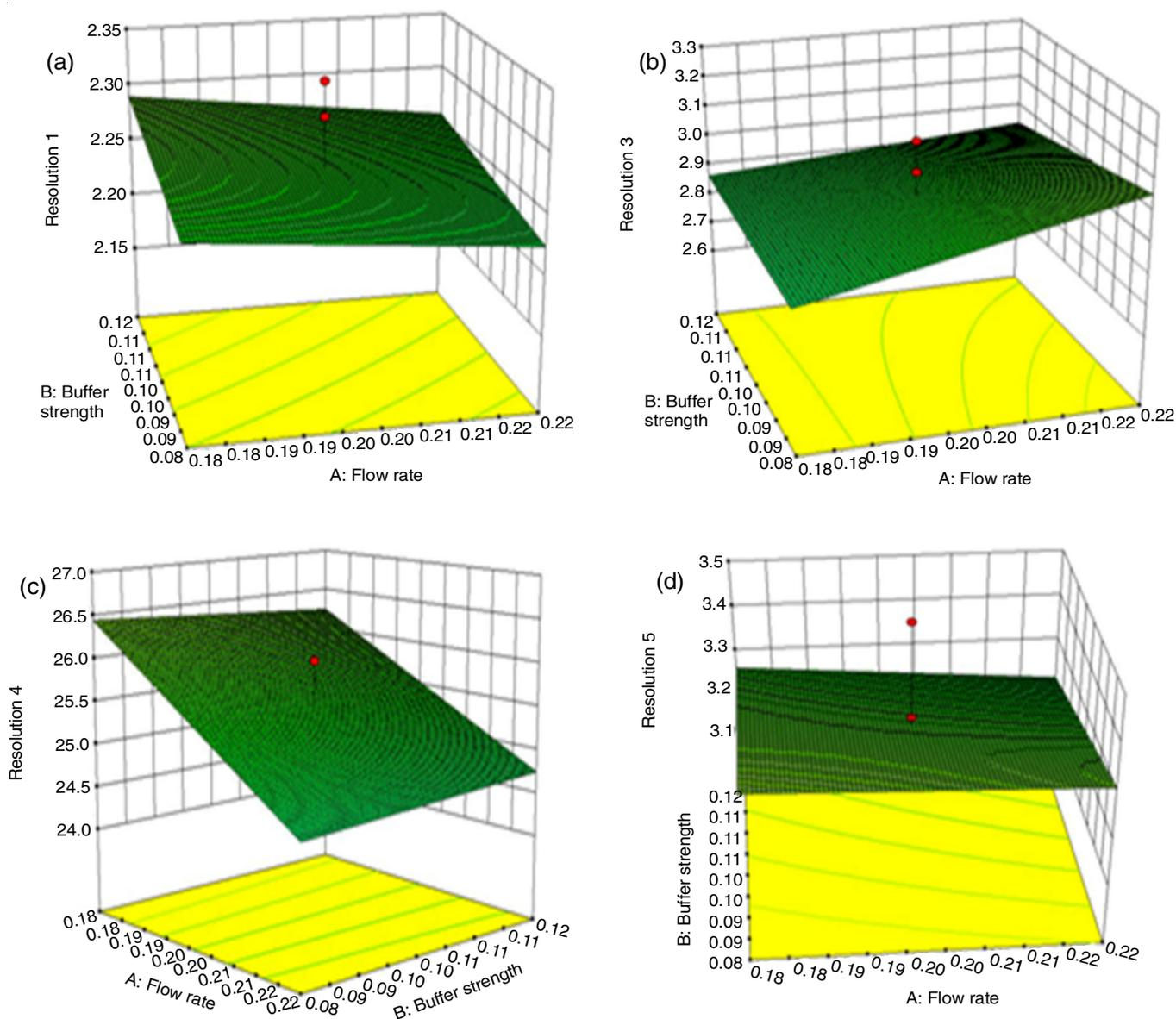
Fig. 4. (a-d): Response surfaces obtained maintaining one variables at the central level and plotting resolution against flow rate and buffer strength (resolution 1 (between impurity B and spironolactone), resolution 3 (between impurity A and impurity D), resolution 4 (between impurity D and impurity C), resolution 5 (between impurity C and impurity E))
