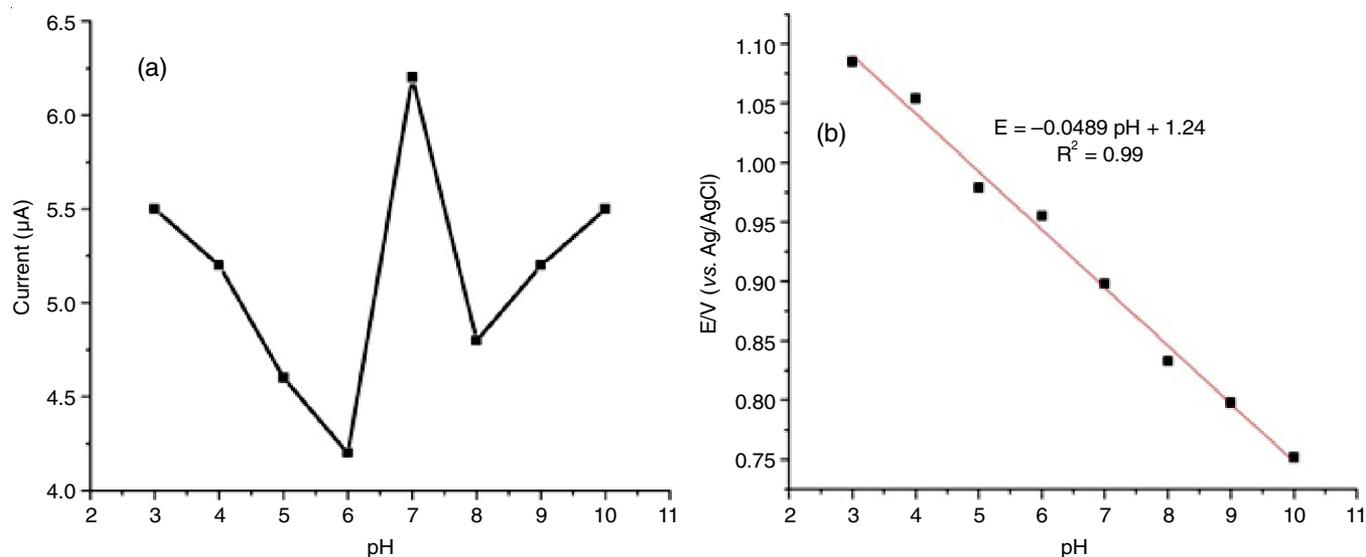
Fig. 5. (a) Cyclic voltammetry of 0.1 mM morphine at poly (CTAB)/GCE in PBS with different pH values (3-10) at scan rate 100  $\text{mV s}^{-1}$  (b) Plot of pH vs.  $E_{pa}$
