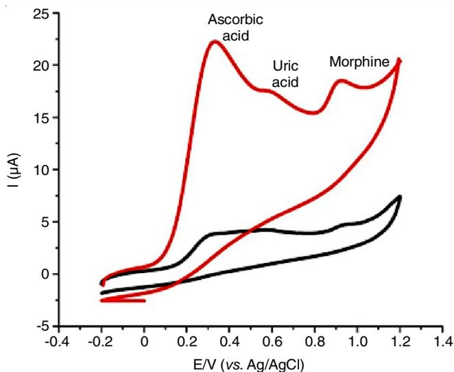
Fig. 8. Cyclic voltammetry of bare and poly (CTAB)/GCE for a mixture of morphine (0.1 mM), ascorbic acid (1 mM) and uric acid (0.2 mM) PBS buffer pH 7 at a scan rate  $100 \text{ mV s}^{-1}$
