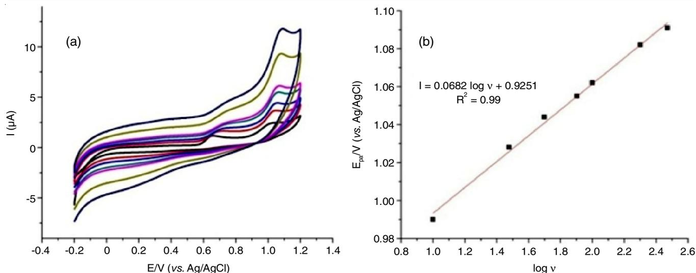
Fig. 6. (a) Cyclic voltammetry of 0.1 mM morphine in 0.1 M (pH 7) PBS at poly(CTAB)/GCE at different scan rates from 10 to 300  $\text{mV s}^{-1}$  (b) Plot of  $\log v$  vs.  $E_p$
