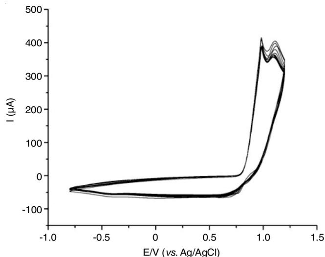
Fig. 1. Cyclic voltammogram of electro-polymerization of CTAB at scan rate 100  $\text{mV s}^{-1}$  at a potential of -1 to 1.4 V for 10 cycles in 0.1 M  $\text{H}_2\text{SO}_4$
