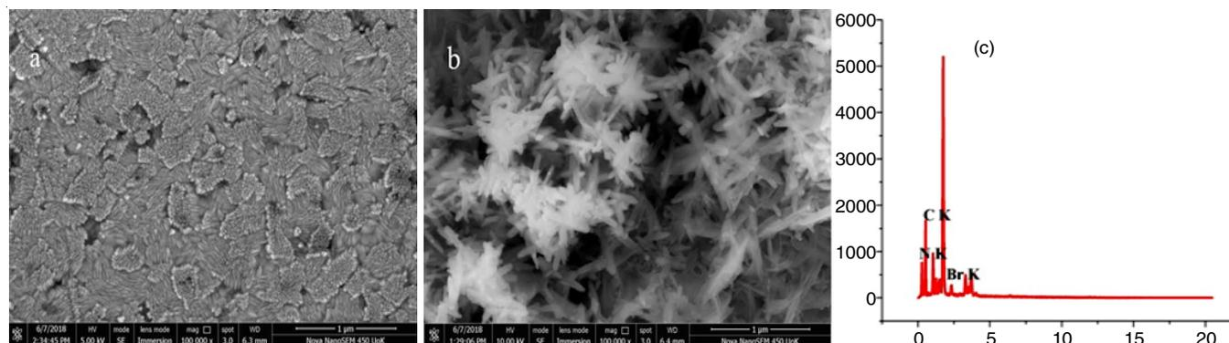
Fig. 2. FESEM images of (a) bare GCE (b) poly(CTAB) (c) energy dispersive X-ray (EDX) spectrum of poly(CTAB)
