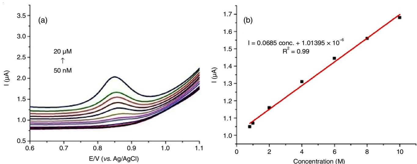
Fig. 7. (a) Differential pulse voltammograms of morphine at different concentrations 50 nM to 20  $\mu\text{M}$  (b) Calibration graph of morphine
