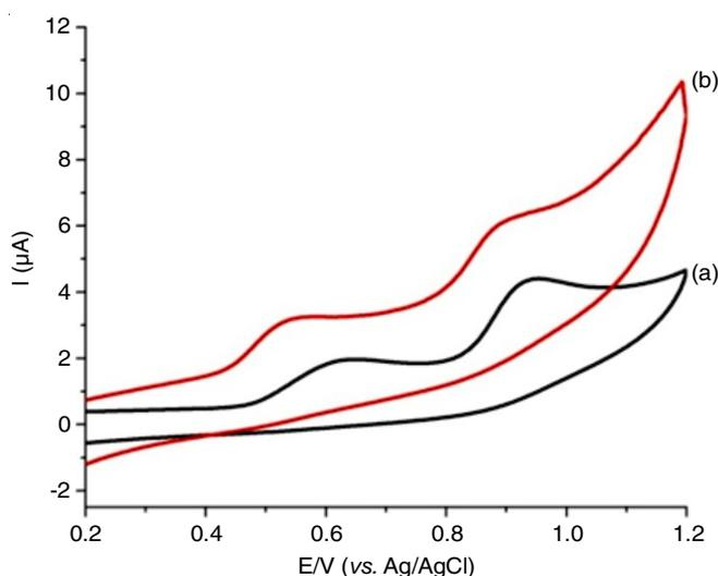
Fig. 4. Cyclic voltammetry of 0.1 mM morphine in 0.1 M (pH 7) PBS at (a) bare GCE (b) poly(CTAB)/GCE
