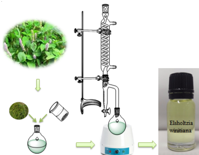
Fig. 1. Process of E. winitiana var. dongvanensis essential oil extraction by hydro-distillation
