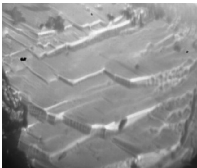
Fig. 9. Etch pattern of urea phosphoric acid crystal with water as an etchant
