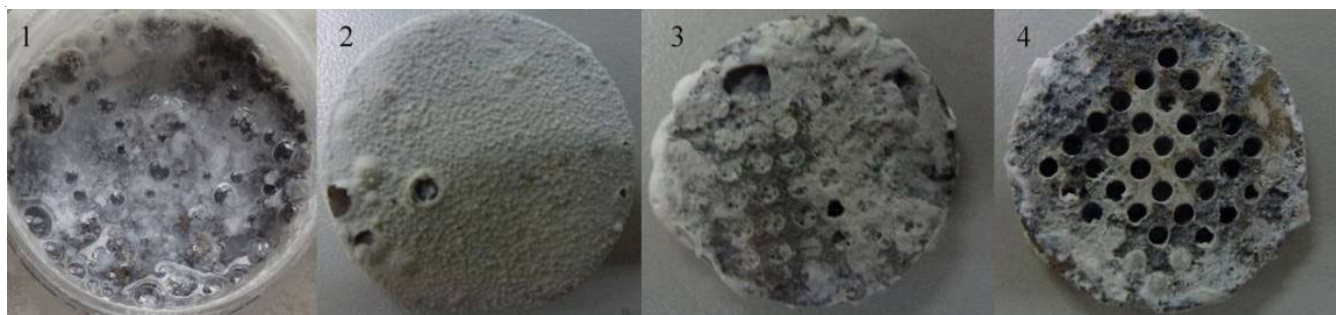
Fig. 4. Optical pictures of samples: 1. AZ31; 2. PDLLA-AZ31-ZnP; 3. PDLLA-porous-1; 4. PDLLA-porous-2 after 3 months
