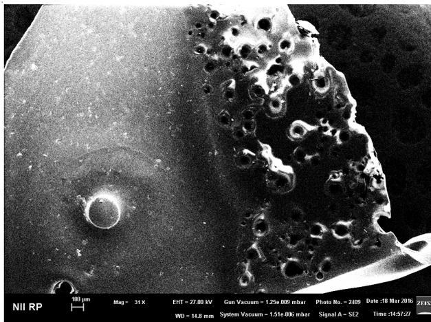
Fig. 4. Scanning electron microscopy of uncrosslinked polyacrylic acid
