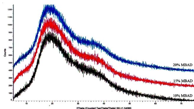
Fig. 3. X-ray phase spectrums of polyacrylic acid crosslinked with methylene-*bis*-acrylamide in different % ratios
