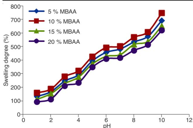
Fig. 2. Dependence curves with swelling rate of crosslinked polyacrylic acid in different ratio pH of environment
