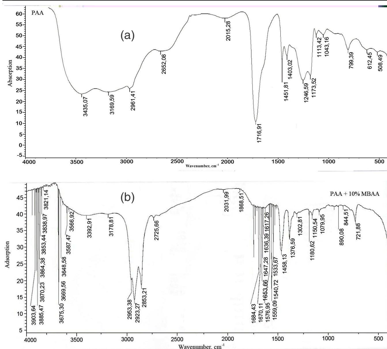
Fig. 1. IR spectrums of polyacrylic acid (a) and hydrogel based on poly-acrylic acid crosslinked with 10 % methylene-bis-acrylamide (b)
