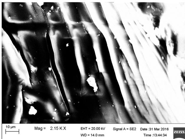
Fig. 5. Scanning electron microscopy of polyacrylic acid crosslinked with methylene-*bis*-acrylamide
