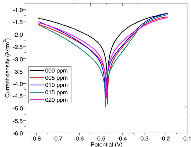
Fig. 2. Tafel plots for mild steel with different concentration of *Schreabera swietenioids* in 1 N HCl
