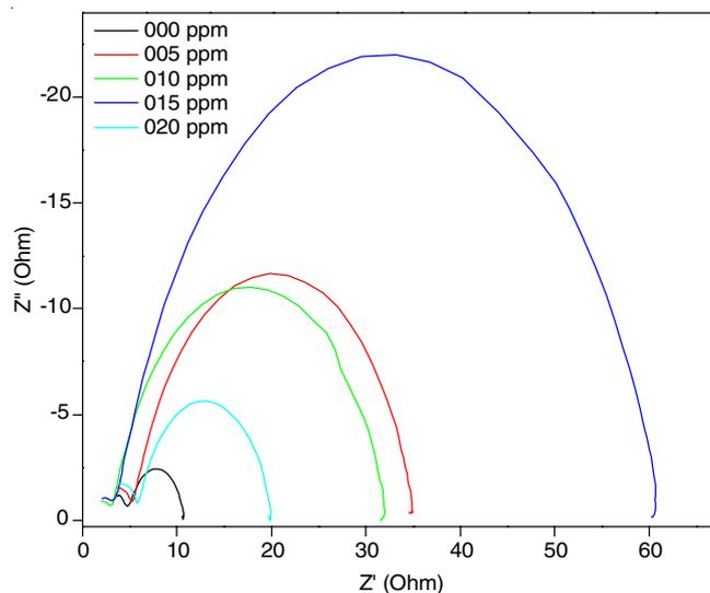
Fig. 3. Nyquist plots of mild steel in absence and presence of different concentration of extract in 1 N HCl
