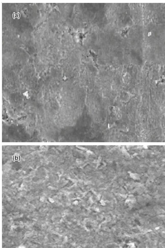
Fig. 4. SEM micrographs of mild steel surface (a) in blank 1 N HCl (b) in the presence of *Schreabera swietenioids* extract
