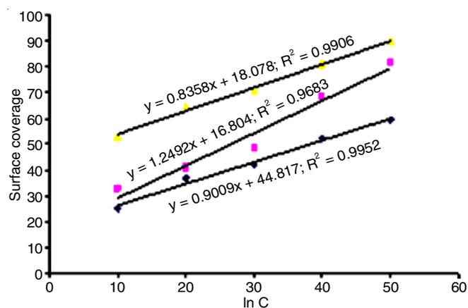
Fig. 5. Temkin isotherm for the *Schreabera swietenioids* extract on the surface of mild steel in 1 N HCl
