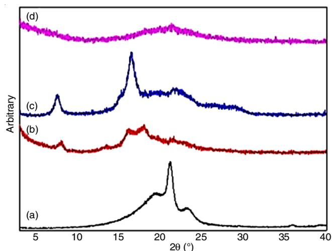
Fig. 5. Wide angle X-ray diffraction patterns of (a) PEDV, (b) PEDV-*g*-poly(*tert*-butylstyrene) (c) PEDV-*g*-poly(*p*-methylstyrene) and (d) PEDV-*g*-poly(styrene)
