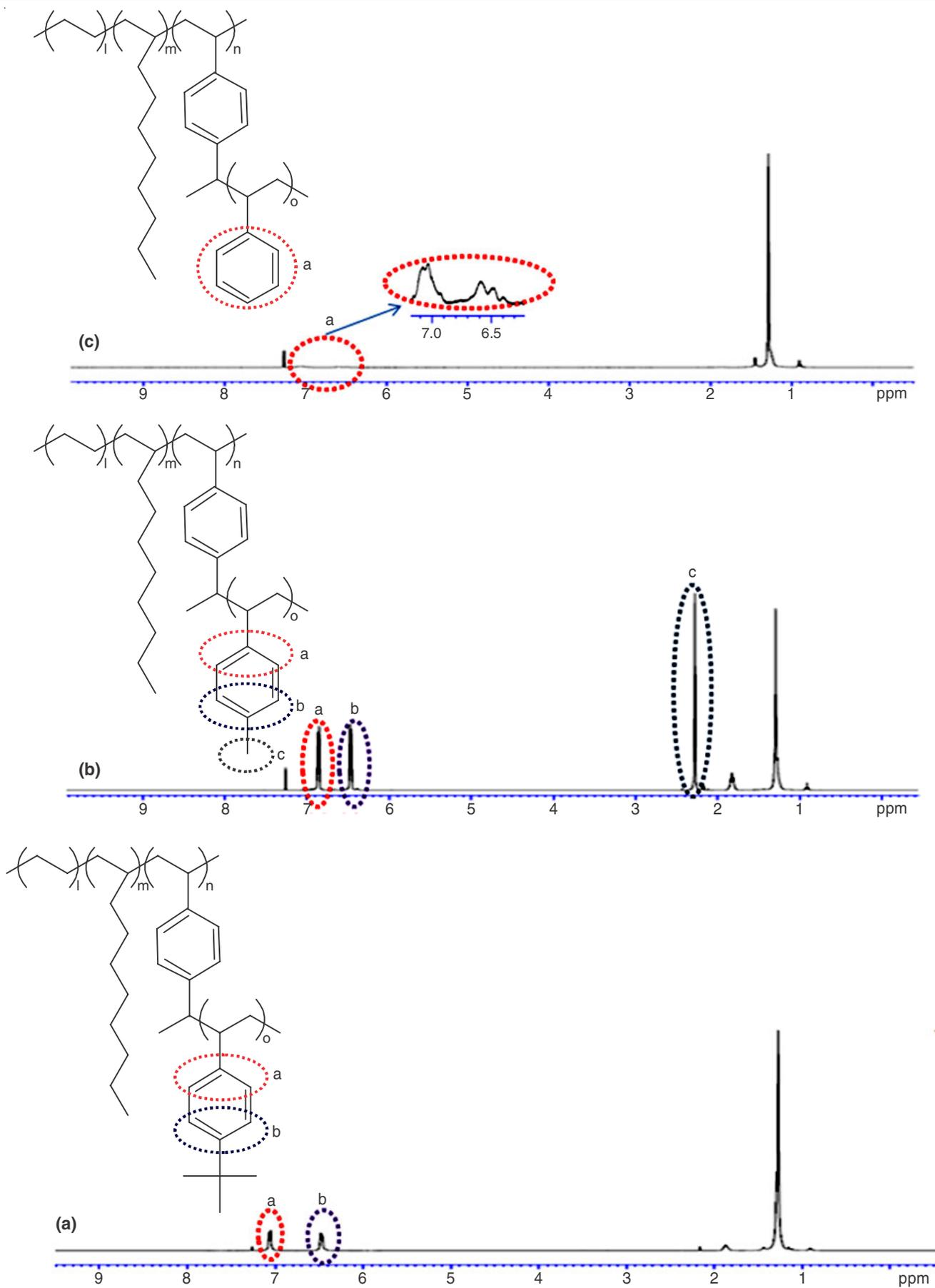
Fig. 3.  $^1\text{H}$  NMR spectra for (a) PEDV-g-poly(*tert*-butylstyrene) (Run 20), (b) PEDV-g-poly(*p*-methylstyrene) (Run 19) and (c) PEDV-g-polystyrene (Run 17)
