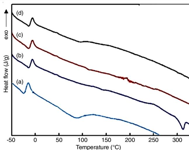
Fig. 4. DSC heating thermograms of (a) PEDV, (b) PEDV-*g*-poly(*tert*-butylstyrene), (c) PEDV-*g*-poly(*p*-methylstyrene) and (d) PEDV-*g*-poly(styrene)
