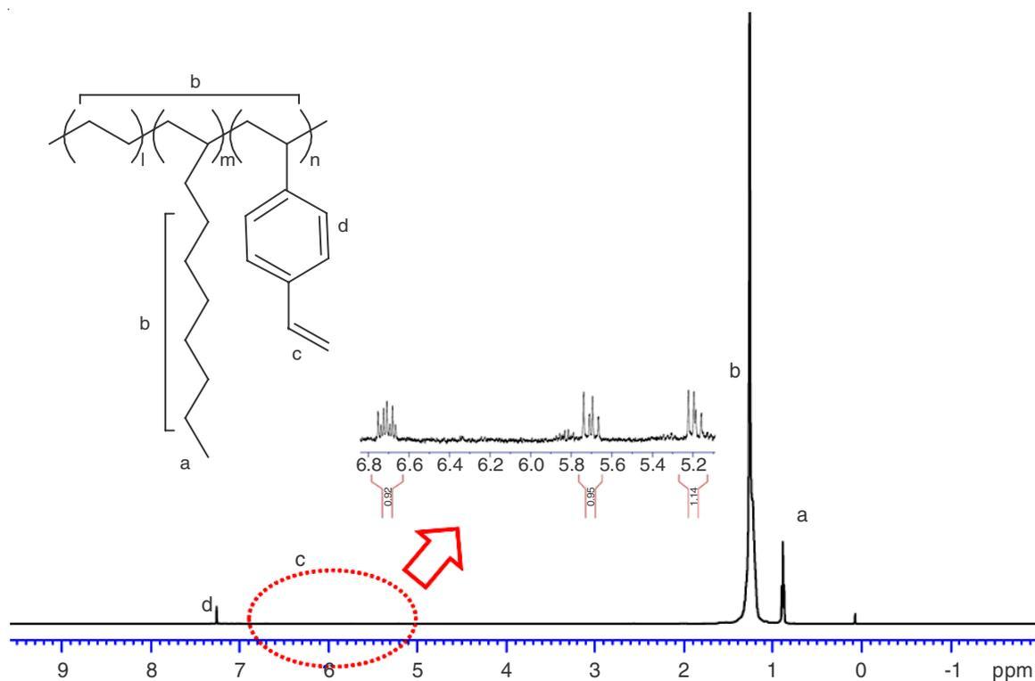
Fig. 1.  $^1\text{H}$ NMR spectrum for PEDV (Run 4)
