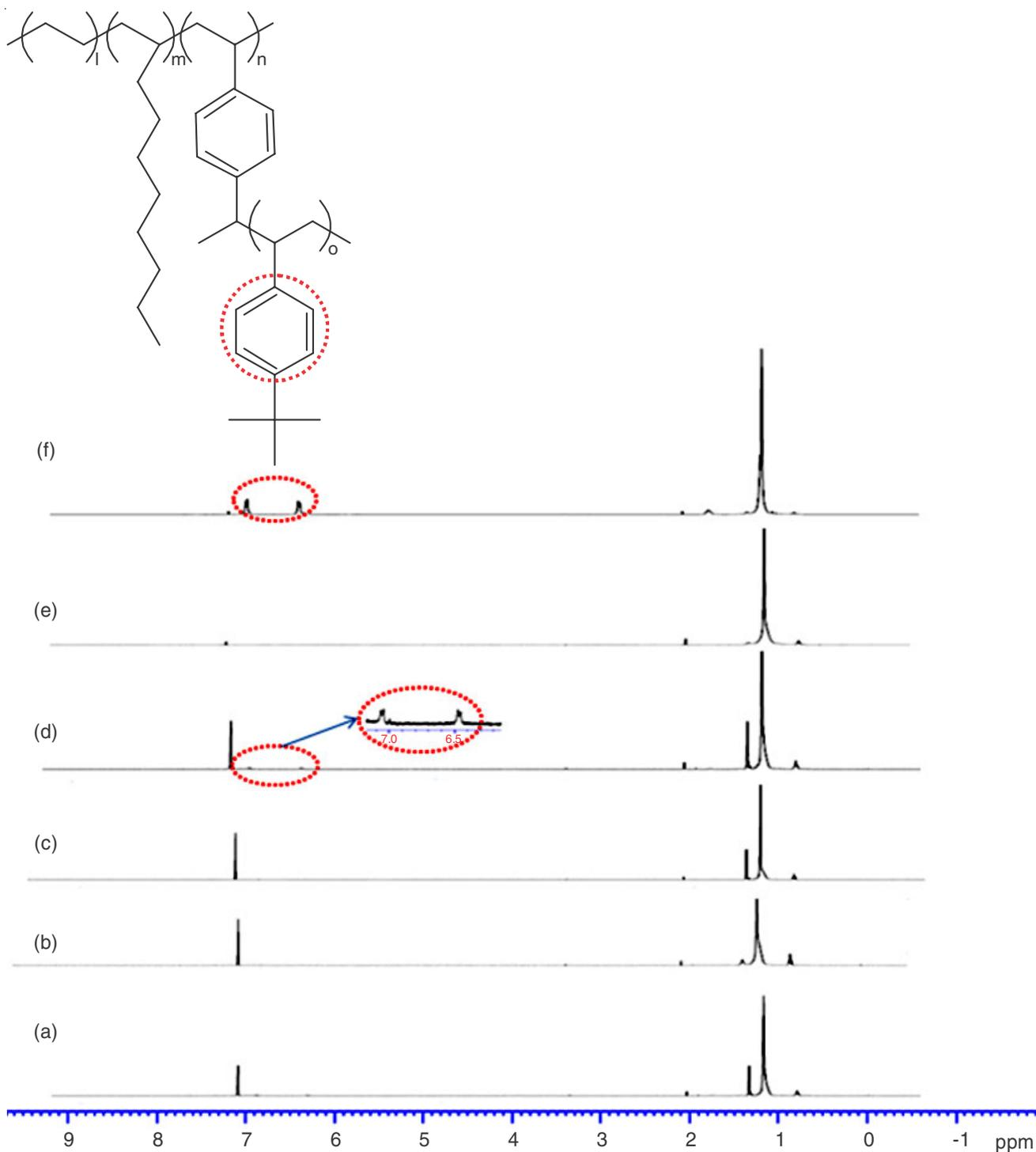
Fig. 2. <sup>1</sup>H NMR spectra for PEDV and PEDV-*g-tert*-butylstyrene: (a) Run 4, (b) Run 8, (c) Run 9, (d) Run 10, (e) Run 11 and (f) Run 12
