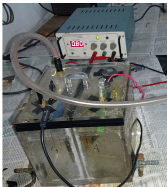
Fig. 3. Microbial electrolysis cell in operation with an electrode spacing of 4cm and electrode potential of 0.8 V
