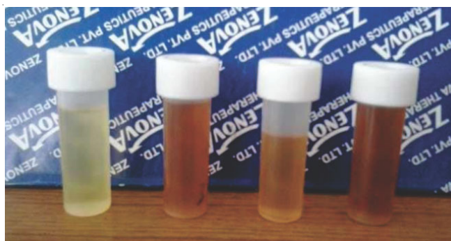
Fig. 2. Biodiesel samples for analysis A, B, A*, B* (A – Fresh sample, B – Sample after 6 months, A* - Fresh sample + 250 ppm BHT and B* - Sample + 250 ppm BHT after 6 months)
