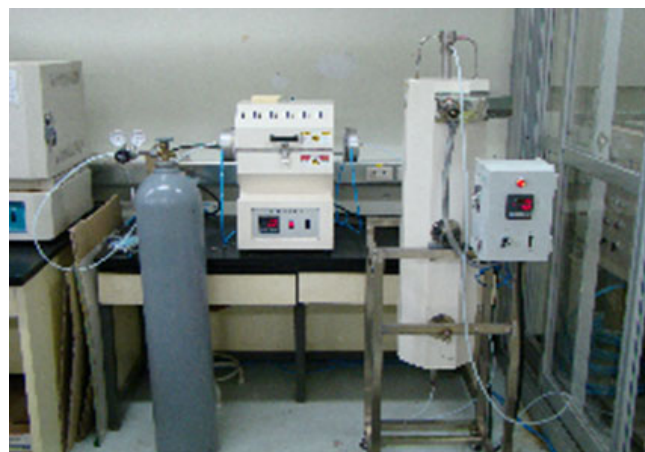
Fig. 1. Schematic diagram and image of the carbonization equipment for the sewage sludge
