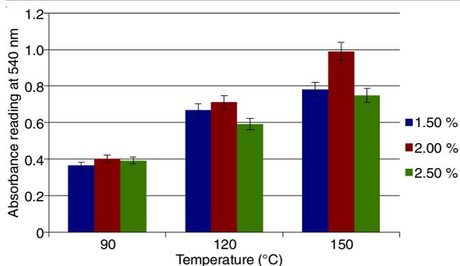
Fig. 2. Absorbance reading obtained from cogon grass that pretreated with 1.5, 2.0 and 2.5 % (w/v) sodium hydroxide at 90, 120 and 150 °C
