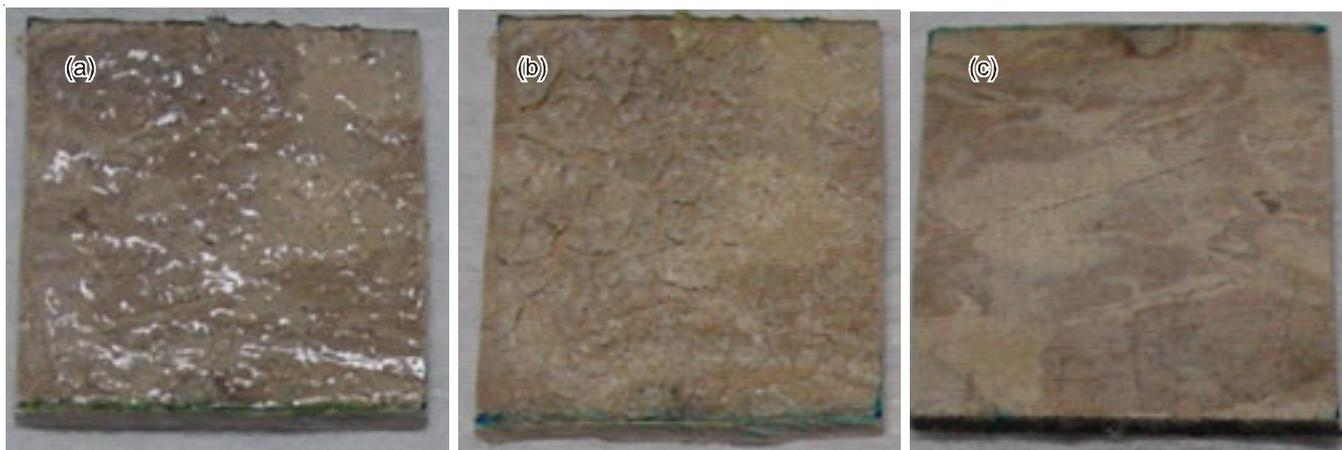
Fig. 6. Optical images of the surfaces (a) before drying, (b) after drying and (c) after detachment of decontamination chemical gel
