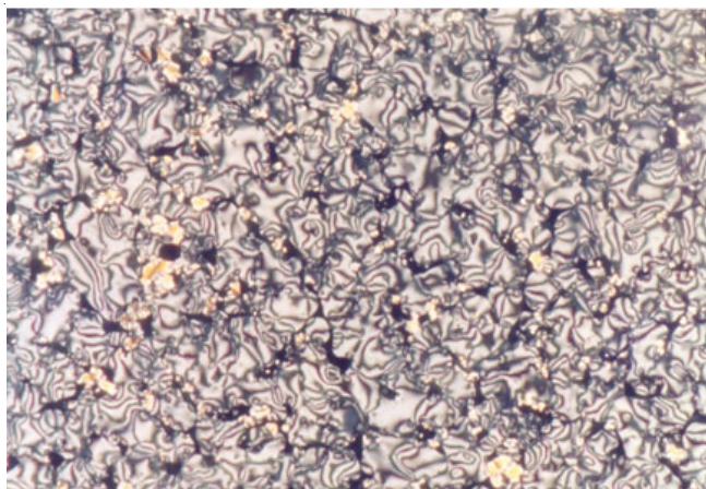
Fig. 1. Polarizing optical micrographs (magnification \times 320 ) of compound 4B in N texture obtained after cooling from isotropic phase to 0 °C
