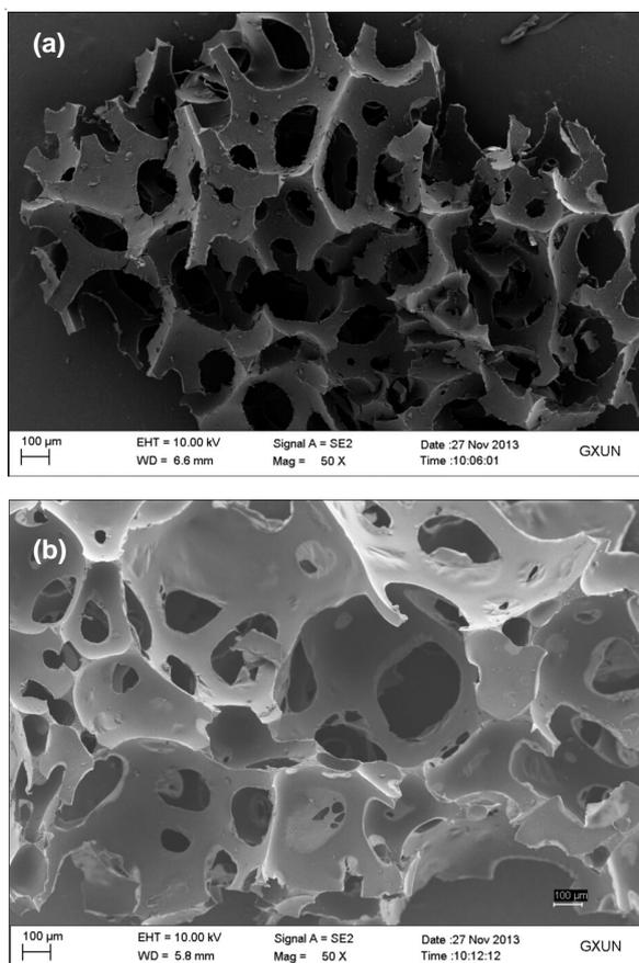
Fig. 6. Bubble figures with different catalyst systems measured by FESEM; (a) The pore structure of foam under the catalysis of  $\text{NdCl}_3$  Schiff Base complex and triethylene diamine catalysis; (b) The pore structure of foam under the catalysis of stannous caprylate and triethylene diamine
