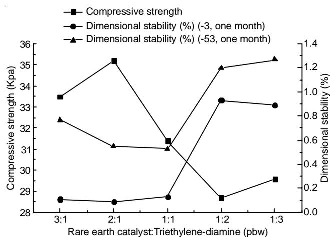
Fig. 5. Effect of catalyst on mechanical properties of foam products
