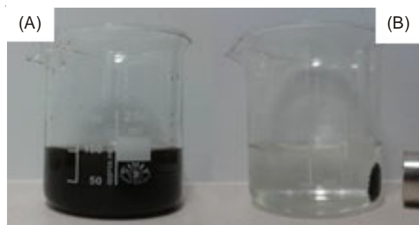
Fig. 1. Demonstration of magnetic iron oxide nanoparticles: (a) magnetic particles dispersed in water (b) their retention towards magnet
