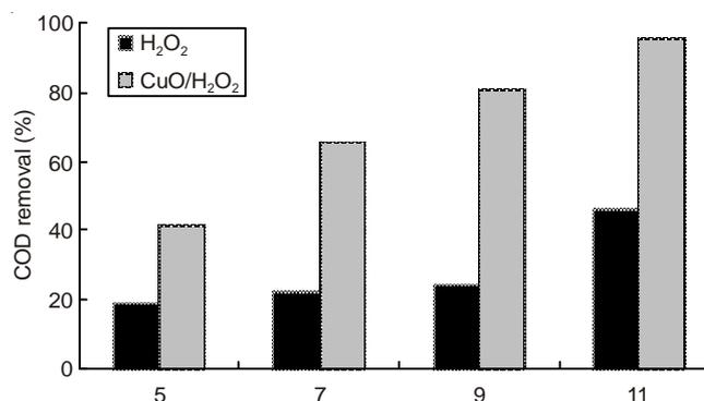
Fig. 3. Effect of pH on antibiotic wastewater degradation
