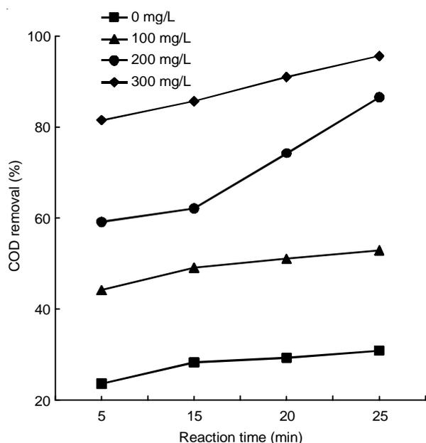
Fig. 1. Effect of catalyst dose on antibiotic wastewater degradation
