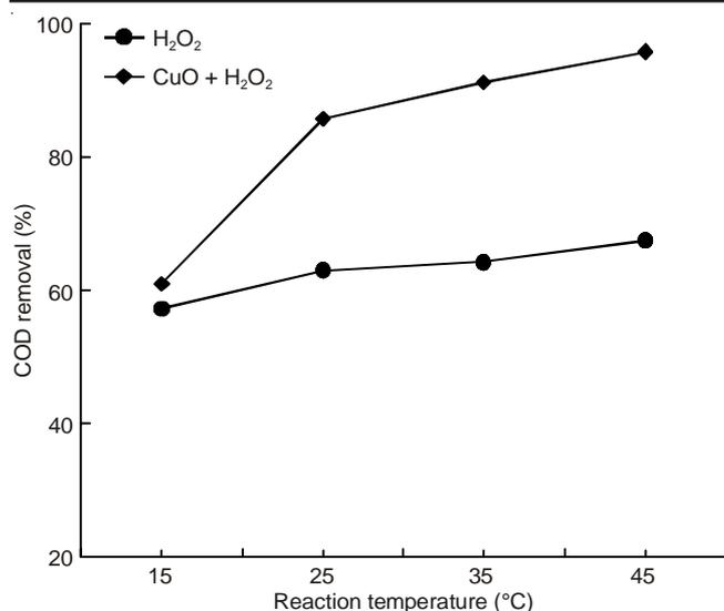
Fig. 4. Effect of temperature on antibiotic wastewater degradation
