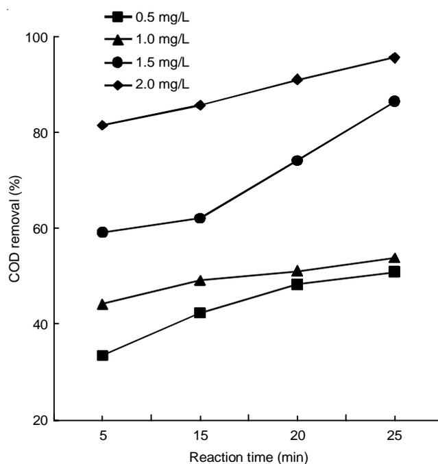
Fig. 2. Effect of hydrogen peroxide dose on antibiotic wastewater degradation
