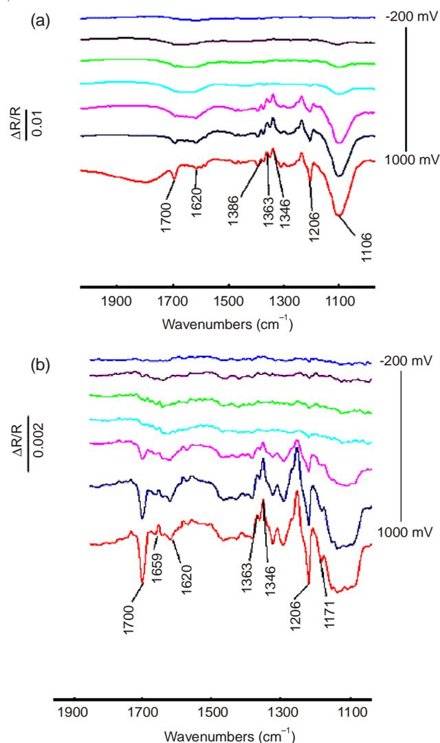
Fig. 3. *in situ* FT-IR spectra collected during electrooxidation of 10 mM benzyl alcohol with TEMPO in the absence (a) and presence (b) of 2,6-lutidine
