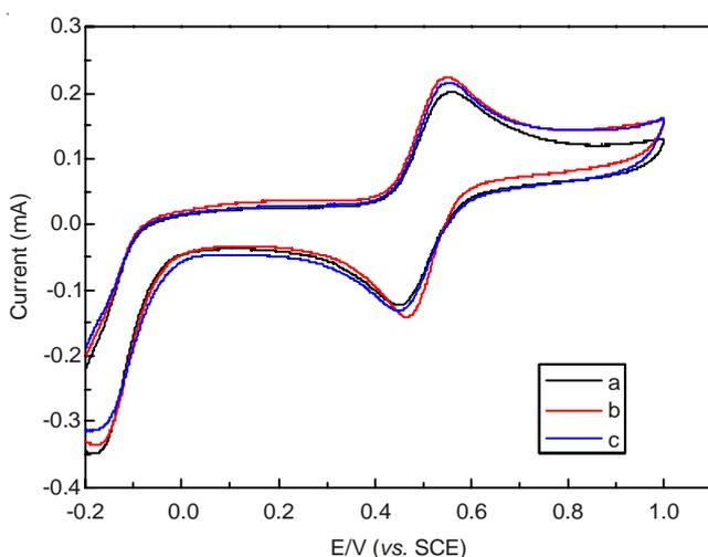
Fig. 1. Cyclic voltammograms of electrooxidation of benzyl alcohol on platinum electrode in  $\text{CH}_3\text{CN}/\text{H}_2\text{O}$  solution containing TEMPO and  $\text{NaClO}_4$ ; (a) blank solution; (b) in the presence of benzyl alcohol ( $10\text{ mM}$ ); (c) in the presence of benzyl alcohol ( $10\text{ mM}$ ) and 2,6-lutidine ( $20\text{ mM}$ )
