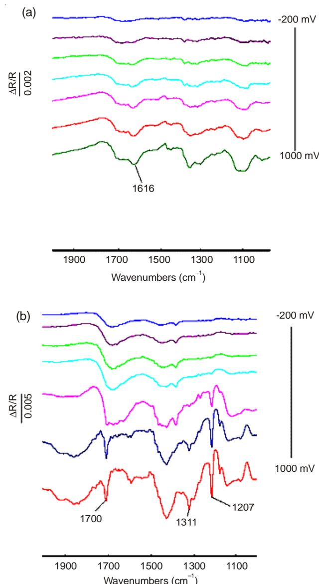
Fig. 4. *in situ* FT-IR spectra collected during oxidation of benzyl alcohol in CH<sub>3</sub>CN/H<sub>2</sub>O solution with benzyl alcohol, 2,6-lutidine and Na<sub>2</sub>CO<sub>3</sub> in the absence (a) and presence (b) of TEMPO
