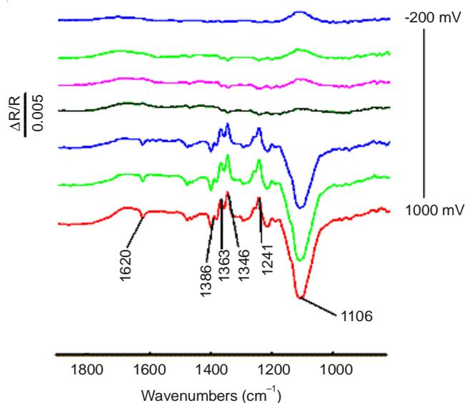
Fig. 2. *in situ* FT-IR spectra collected during electrochemical oxidation of TEMPO on platinum electrode in  $\text{CH}_3\text{CN}/\text{H}_2\text{O}$  solution containing TEMPO and  $\text{NaClO}_4$
