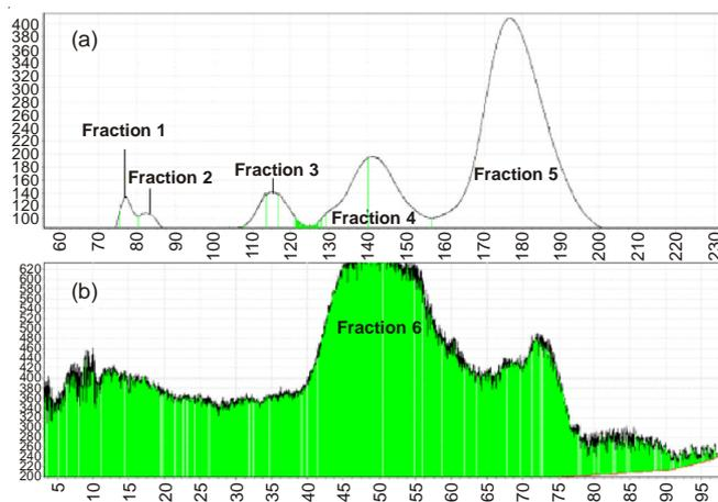
Fig. 1. HSCCC of sub-fraction FC. (a): the HSCCC apparatus was run in forward rotation model; (b): the forward rotation model was converted to the reverse rotation mode 230 min after the sample injection
