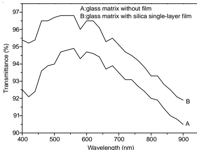
Fig. 1. Transmittance of the glass matrix and the silica single-layer film
