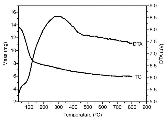
Fig. 4. TG and DTA curves of the silica single-layer film
