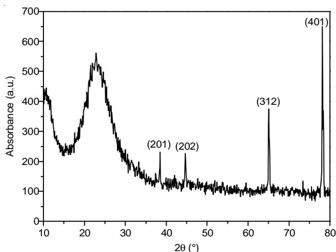
Fig. 3. X-Ray diffraction patterns of the silica single-layer film
