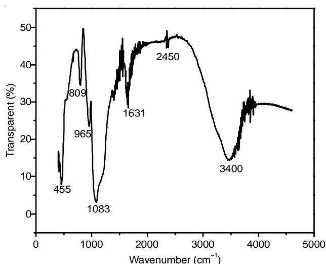
Fig. 2. FTIR spectra of the silica single-layer film
