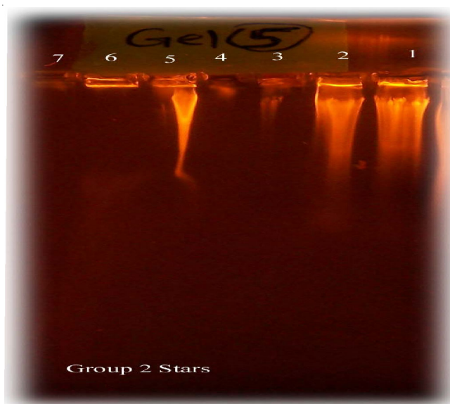
Fig. 5. Electrophoretic mobility of Calf thymus DNA treated with H_3AHMP (lane 1), ligand with DNA (lane 2), ligand with DMSO (lane 3), Fe complex (lane 4), Mn complex (lane 5), Cr complex (lane 6), Cd complex and (lane 7), for Zn complex
