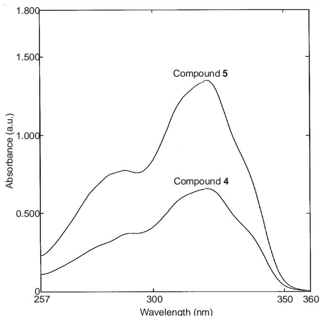
Fig. 1. Adsorption spectra of dendrimers having cyclam core compounds 4 and 5 in  $\text{CH}_2\text{Cl}_2$
