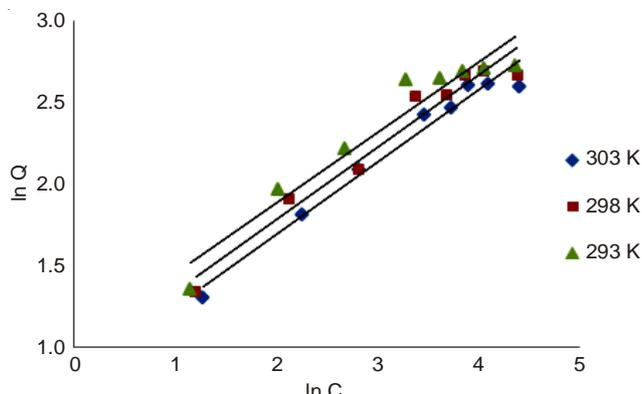
Fig. 6. Linear fitting of the Freundlich isotherm for  $Cd^{2+}$  onto *Agaricus blazei* Murill at different temperature
