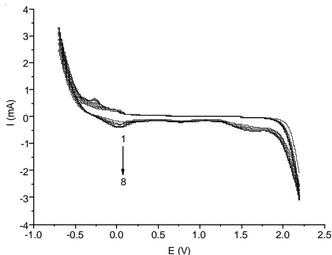
Fig. 1. Cyclic voltammograms of the palladium doped L-arginine in the polymerization process at scan rate of 160 mV/s. From 1 to 8 indicate the total number of sweeps
