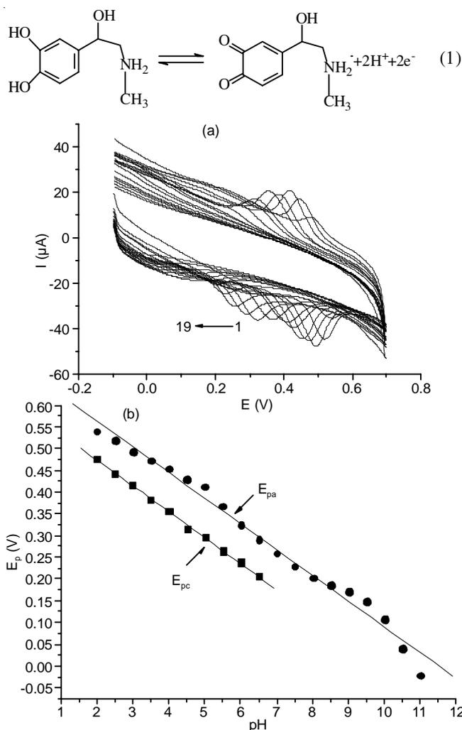
Fig. 4. Cyclic voltammograms of epinephrine at Pd-PLA/GCE at different effects of solution pH (a) and the relationship curve between the peak potential and pH (b); pH from 1 to 19: 2.0, 2.5, 3, 3.5, 4, 4.5, 5, 5.5, 6, 6.5, 7, 7.5, 8, 8.5, 9, 9.5, 10, 10.5, 11; Scan rate: 160 mV/s; epinephrine concentration:  $2.50 \times 10^{-5}$  mol/L
