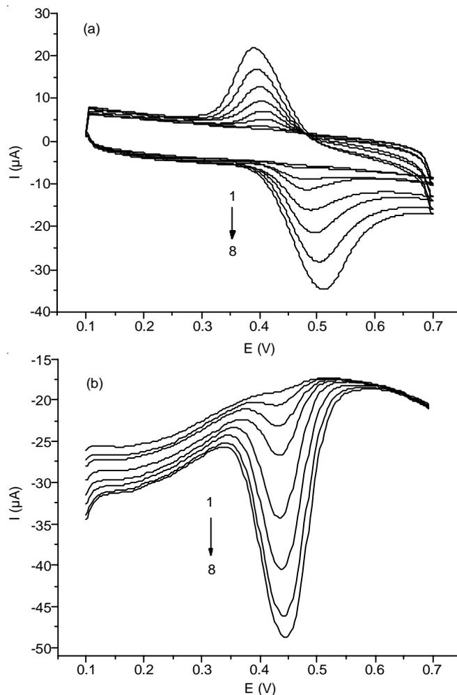
Fig. 8. Cyclic voltammeters curve of epinephrine with different concentrations at Pd-PLA/GCE (a) and differential pulse voltammeters curve of epinephrine with different concentrations at Pd-PLA/GCE (b); epinephrine concentrations (from 1 to 8):  $5 \times 10^{-7}$ ,  $1 \times 10^{-6}$ ,  $5 \times 10^{-6}$ ,  $1 \times 10^{-5}$ ,  $3 \times 10^{-5}$ ,  $5 \times 10^{-5}$ ,  $8 \times 10^{-5}$ ,  $1 \times 10^{-4}$  mol/L
