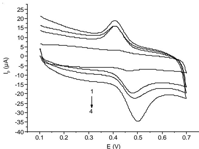
Fig. 3. Cyclic voltammograms of  $2.50 \times 10^{-5}$  mol/L epinephrine at glassy carbon electrode (1), Pd/GCE (2), PLA/GCE (3) and Pd-PLA/GCE (4); PBS: pH = 3; scan rate: 160 mV/s; epinephrine concentration:  $2.50 \times 10^{-5}$  mol/L
