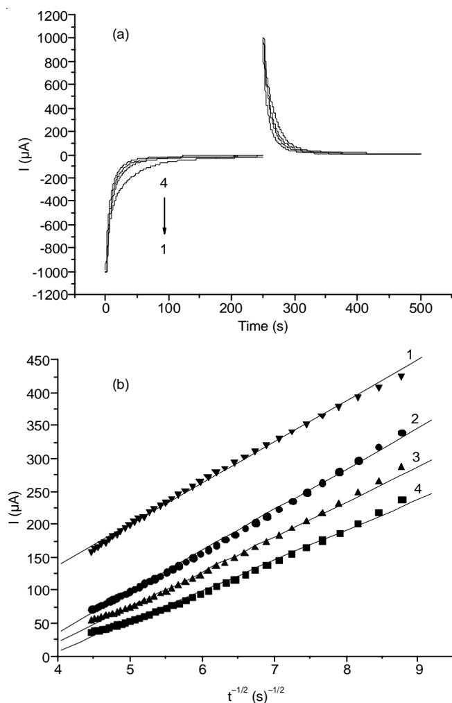
Fig. 7. Chronoamperograms of epinephrine at the different modified glassy carbon electrode (a) and the relationship curve between  $I$  and  $t^{-1/2}$  (b); Pd-PLA/GCE (1); PLA/GCE (2); Pd/GCE (3) and GCE (4); PBS: pH 3; epinephrine concentration:  $2.50 \times 10^{-5}$  mol/L
