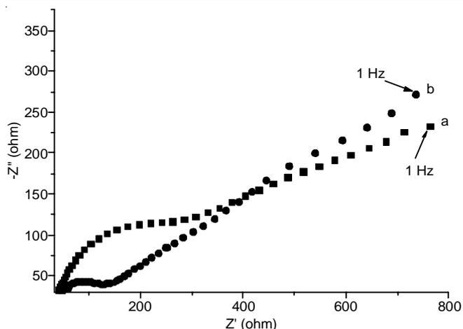
Fig. 2. Nyquist impedance plots of the bare glassy carbon electrode (a) and Pd-PLA/GCE (b) in 0.1 mol/L  $[\text{Fe}(\text{CN})_6]^{3/4-}$  solution containing 0.1 mol/L KCl
