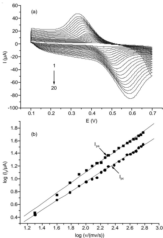
Fig. 5. Cyclic voltammograms of epinephrine at different scan rates (a) and the relationship curve between  $\log I_p$  and  $\log v$  (b); scan rate from 1 to 20: 20, 40, 60, 80, 100, 120, 140, 160, 180, 200, 240, 280, 320, 360, 400, 440, 480, 520, 560 and 600 mV S<sup>-1</sup>; epinephrine concentration:  $2.50 \times 10^{-5}$  mol/L
