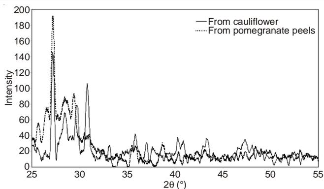
Fig. 3. Powder X-ray diffraction patterns of MgO nanoparticles using water extracts of cauliflower and pomegranate peels
