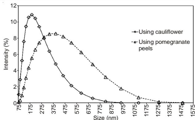
Fig. 4. Influence of source of water extract on hydrodynamic size distribution of dispersions of MgO nanoparticles in water
