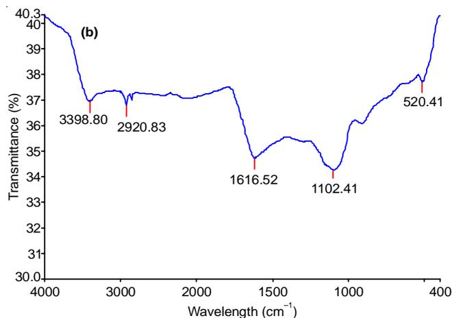
Fig. 6. FTIR spectra of MgO nanoparticles synthesized using [a] water extract of cauliflower; [b] water extract of pomegranate peels
