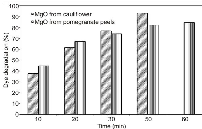
Fig. 8. Photocatalytic activity of green-synthesized MgO nanoparticles under UV irradiation
