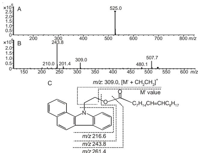
Fig. 3. Mass spectra of oleic acid (C18:1) derivative and its cleavage mode
