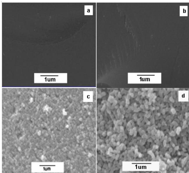
Fig. 1. SEM micrographs of the samples at different heat treatment temperature (a) 500 °C, (b) 530 °C, (c) 550 °C, (d) 580 °C
