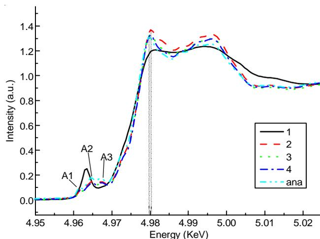
Fig. 4. Ti K-edge XANES of unheat ed and heated treatment samples: ana. = anatase, 1 = unheated, 2 = 500 °C, 3 = 530 °C, 4 = 580 °C
