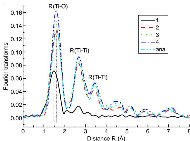
Fig. 5. Fourier transformation curves of Ti K-edge EXAFS of samples: ana. = anatase, 1 = unheated, 2 = 500 °C, 3 = 530 °C, 4 = 580 °C
