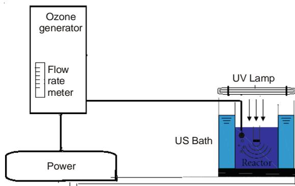
Fig. 1. Diagram of sono-reactor
