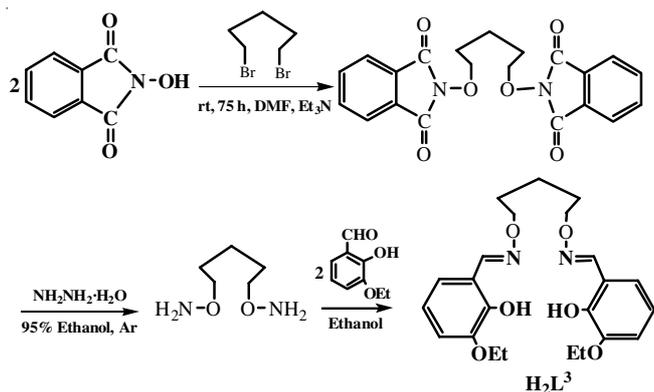
Fig. 3. Synthetic route to the Salamo-type bisoxime  $H_2L^3$
