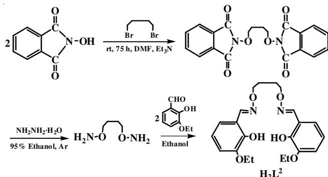
Fig. 2. Synthetic route to the Salamo-type bisoxime  $H_2L^2$
