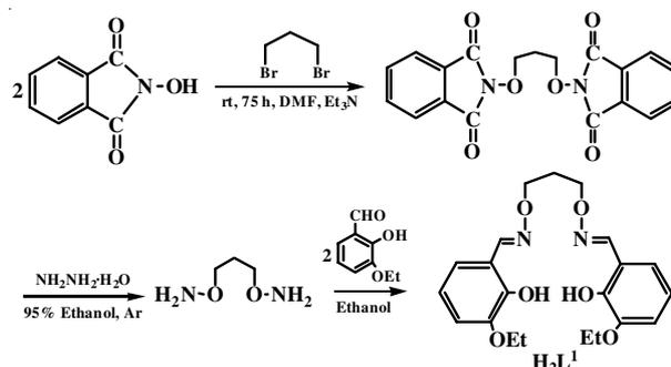
Fig. 1. Synthetic route to the Salamo-type bisoxime  $H_2L^1$
