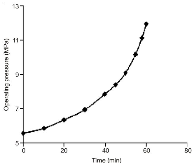
Fig. 5. Changing curve of dish-tube reverse osmosis operating pressure
