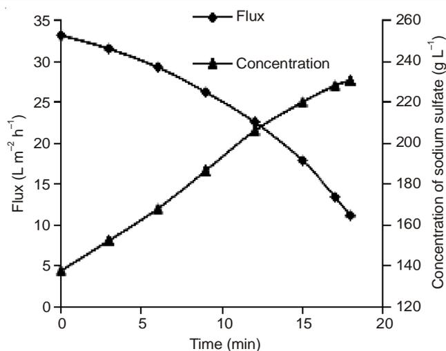
Fig. 6. Changing curve of dish-tube reverse osmosis flux and sodium sulfate concentration
