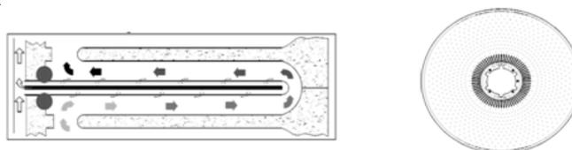
Fig. 2. Schematic of flow channel and hydraulic disc
