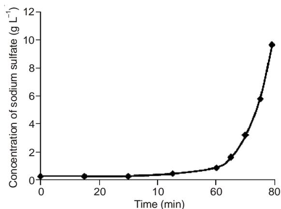
Fig. 7. Changing curve of permeated water sodium sulfate concentration
