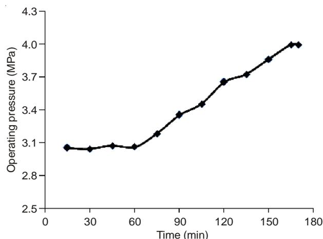
Fig. 4. Changing curve of reverse osmosis operating pressure
