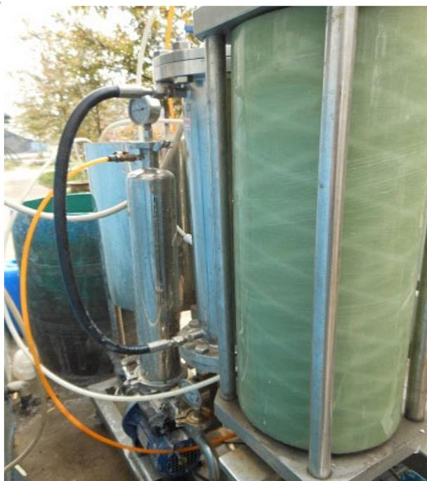
Fig. 3. Dish-tube reverse osmosis testing equipment
