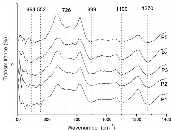
Fig. 1. FTIR spectra of  $(1-x)(0.5P_2O_5-0.25Na_2O-0.25Li_2O)-xLa_2O_3$  glasses
