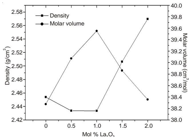
Fig. 2. Composition dependence of density and molar volume for  $(1-x)(0.5\text{P}_2\text{O}_5-0.25\text{Na}_2\text{O}-0.25\text{Li}_2\text{O})-x\text{La}_2\text{O}_3$  glasses
