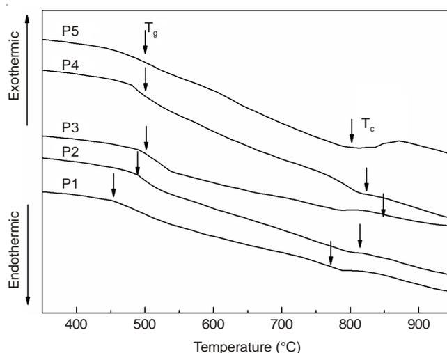
Fig. 3. DTA traces of  $(1-x)(0.5\text{P}_2\text{O}_5-0.25\text{Na}_2\text{O}-0.25\text{Li}_2\text{O})-x\text{La}_2\text{O}_3$  glasses
