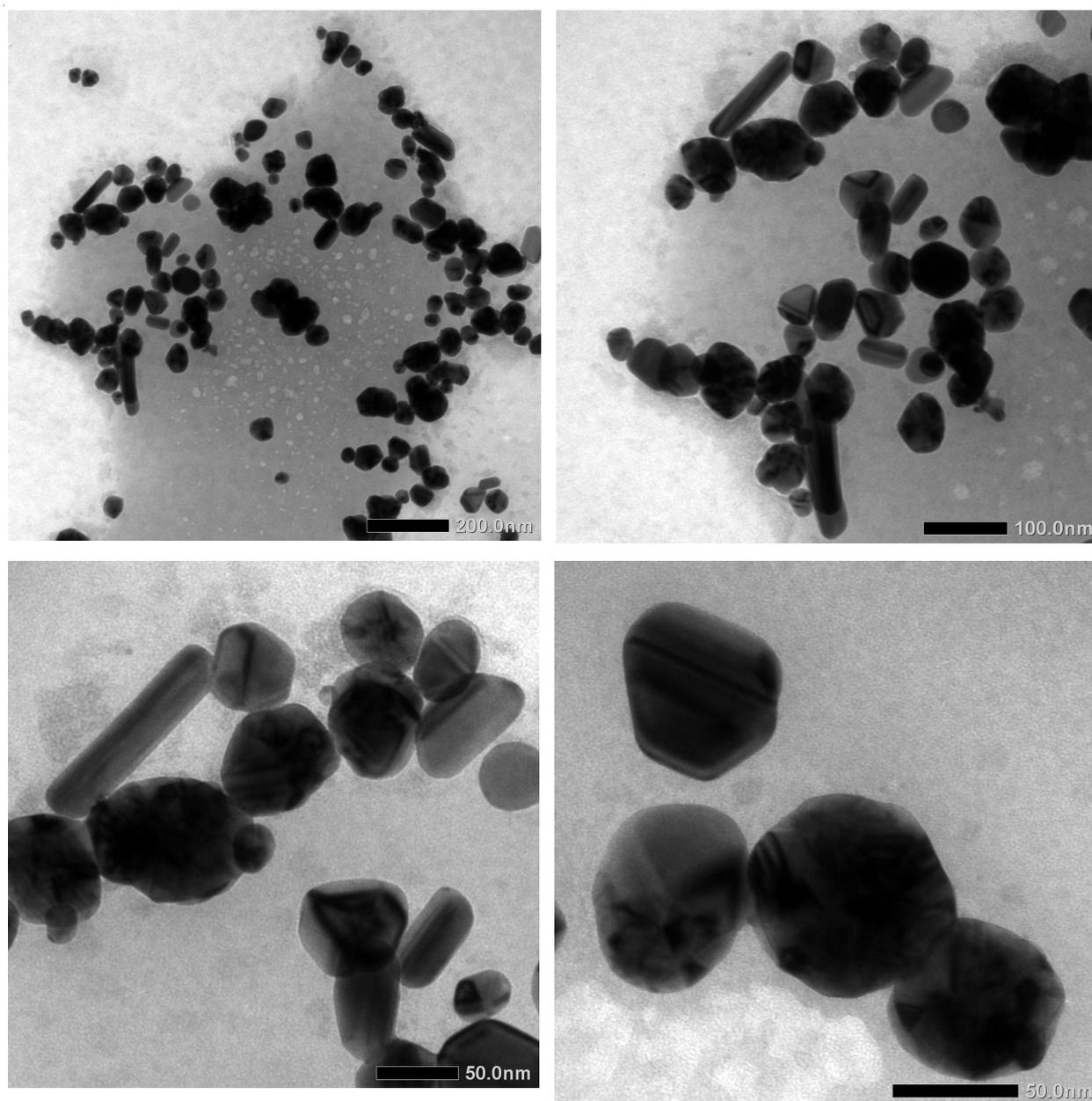
Fig. 6. TEM picture of silver nanoparticles
