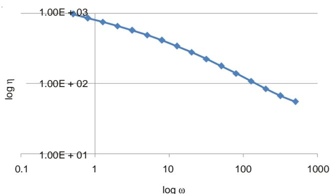
Fig. 8. Angular frequency dependence of complex viscosity of NR1 at 40  $^{\circ}$ C
