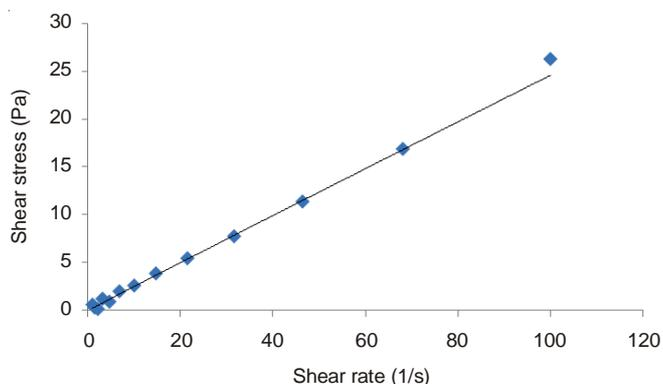
Fig. 6. Fit of Ostwald model for NR4 at 40 °C
