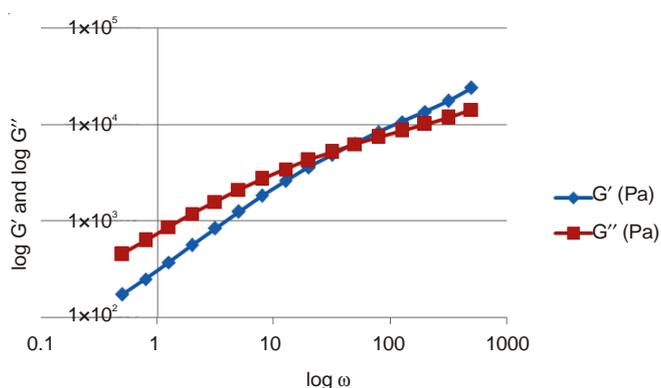
Fig. 9. Angular frequency dependence of dynamic moduli ( $G'$  and  $G''$ ) of NR1 at 40  $^{\circ}$ C
