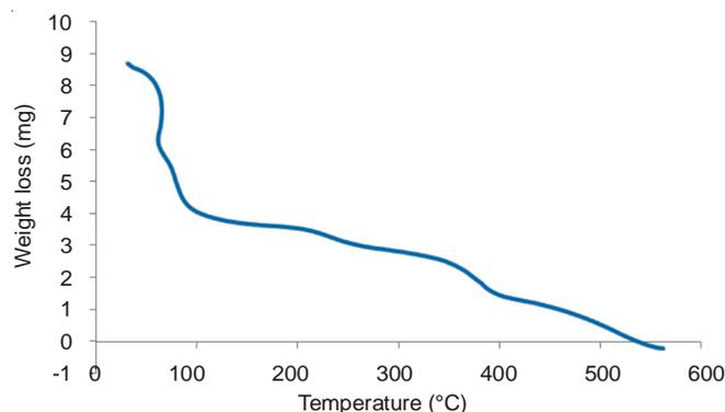
Fig. 1. Thermogravimetric curve of the hydrogel NR4
