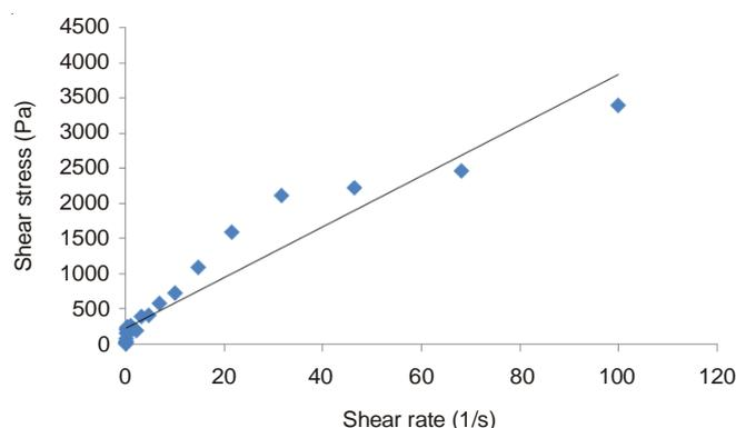
Fig. 7. Fit of Bingham Model for NR2 at 50 °C
