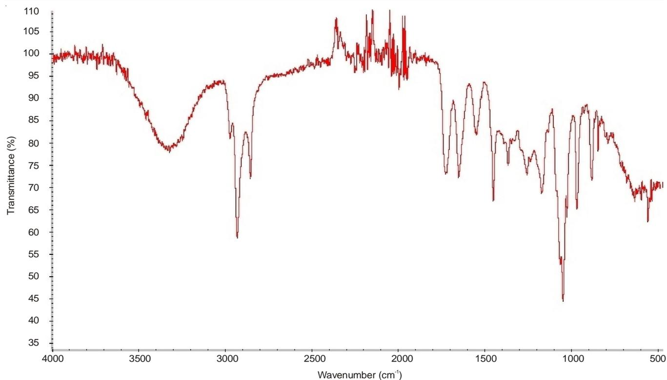
Fig. 2. FTIR spectrum of the gel NR4
