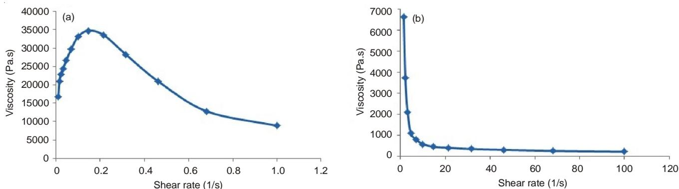
Fig. 4. Rheogram of NR1 at 50 °C (a) at low shear rate (b) at high shear rate
