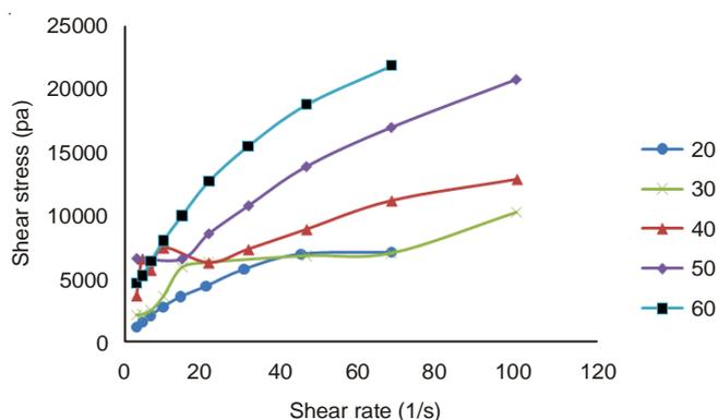
Fig. 3. Graph between shear rate and shear stress for NR1 at 20, 30, 40, 50 and 60 °C
