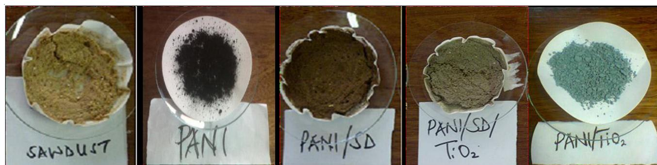
Fig. 1. Appearance of the polyaniline composites synthesized; SD (light brown), polyaniline (PANI) (dark green), PANI/SD (brown), PANI/TiO<sub>2</sub> (light green) and PANI/SD/TiO<sub>2</sub> (light green) after synthesis
