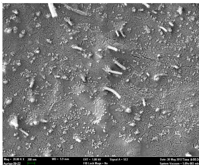
Fig. 3. FESEM images of CNT/FE (the razor cut surface)
