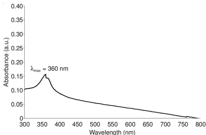
Fig. 1. UV-visible spectrum of the synthesized ZnO nanoparticles
