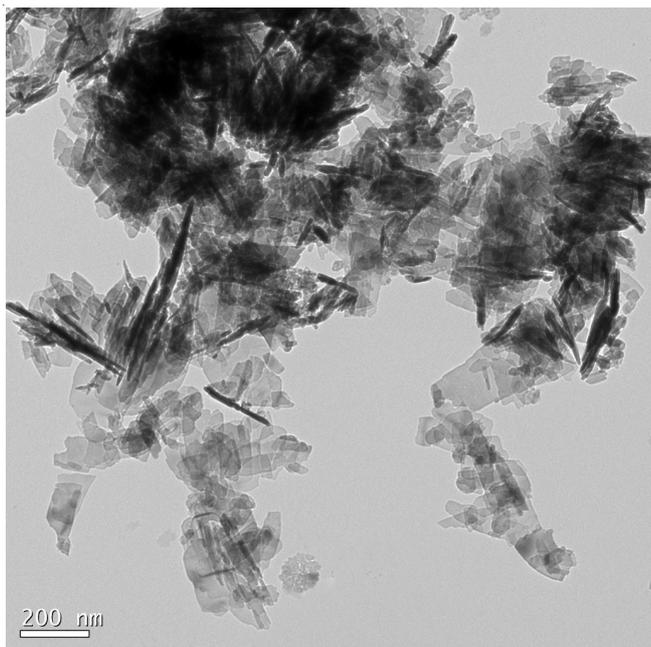
Fig. 3. TEM image of the synthesized ZnO nanoparticles
