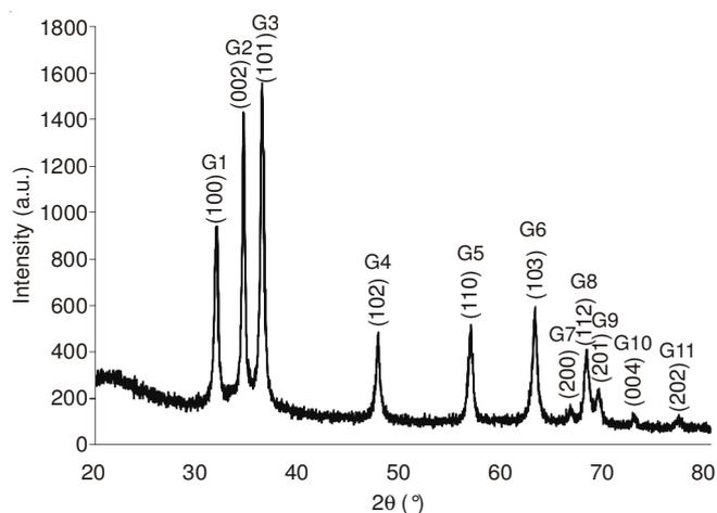
Fig. 2. XRD pattern of the synthesized ZnO nanoparticles
