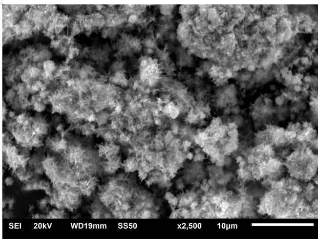
Fig. 4. SEM image of the synthesized ZnO nanoparticles
